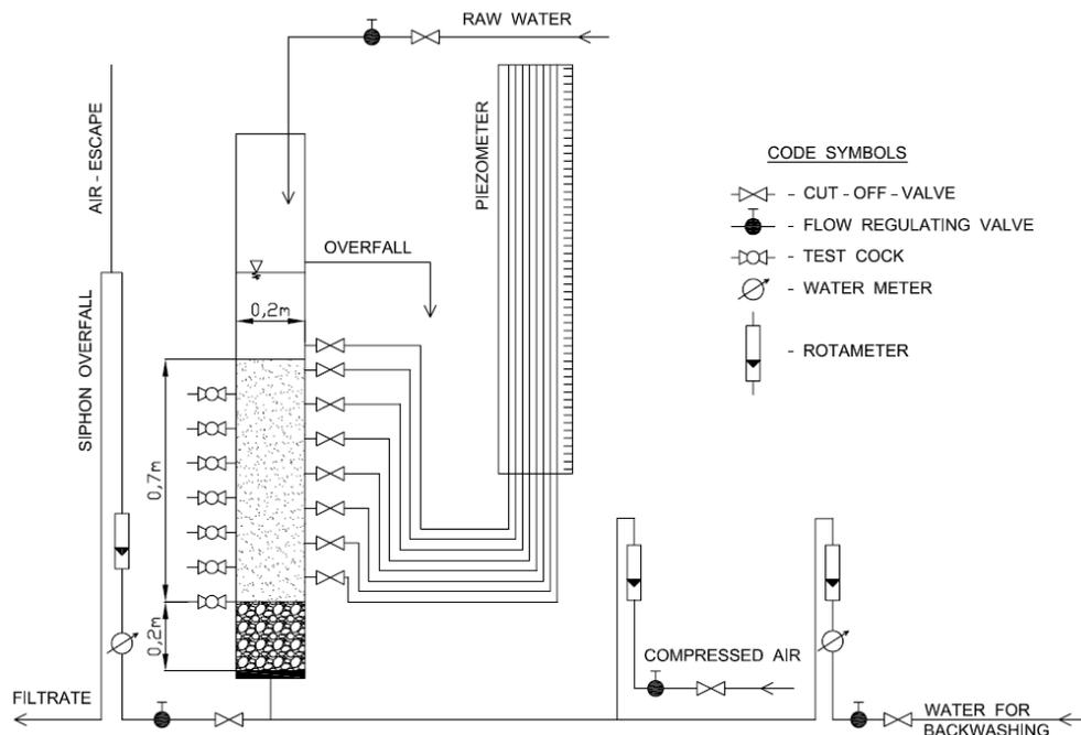
FIGURE 1. The scheme of the testing bench
