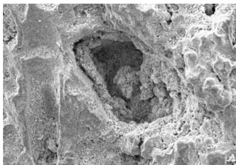
FIGURE 12. The SEM micrograph of the MDMC-3 coat structure
