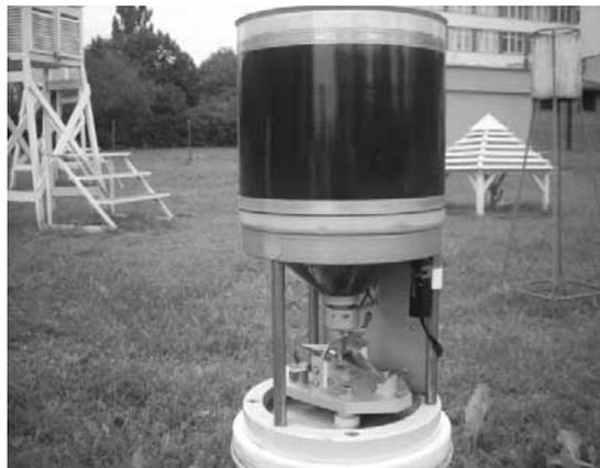
FIGURE 1. Measurement unit in the telepluviometer
