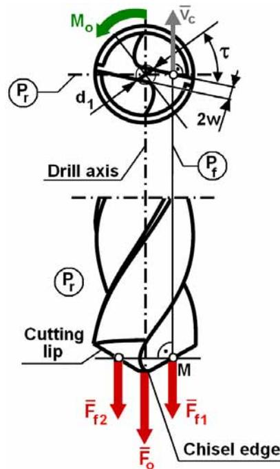
Figure 2. Edge geometry at a cutting point on the lip.
