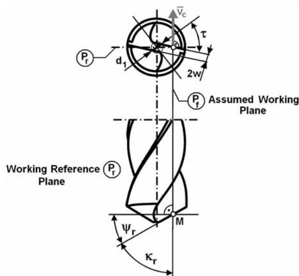
Figure 1. View showing geometric data of a twist drill.
