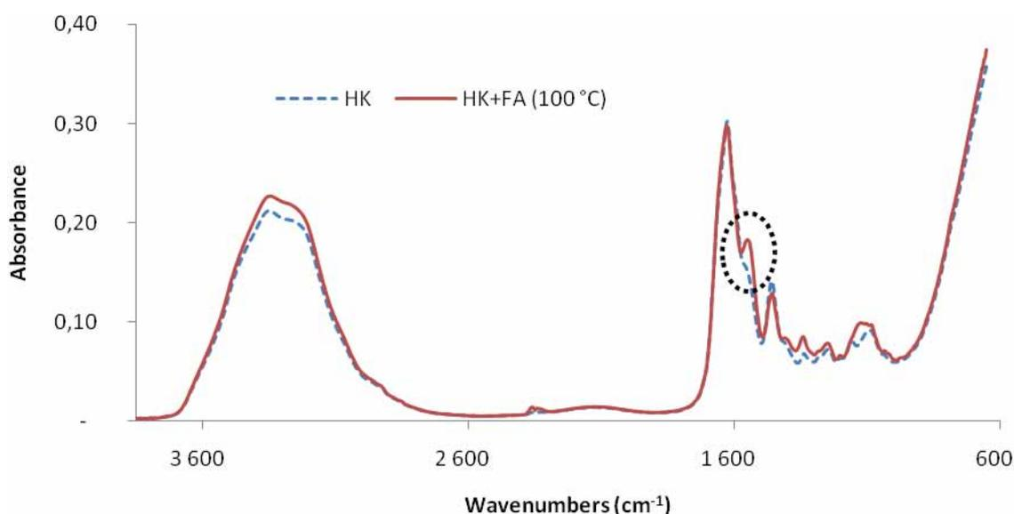
*Fig. 1* FTIR spectrum of collagen hydrolysate after reaction with formaldehyde.
