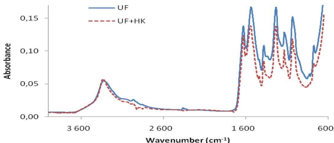
**Fig. 2** FTIR spectrum of UF adhesive and UF adhesive with collagen hydrolysate.
