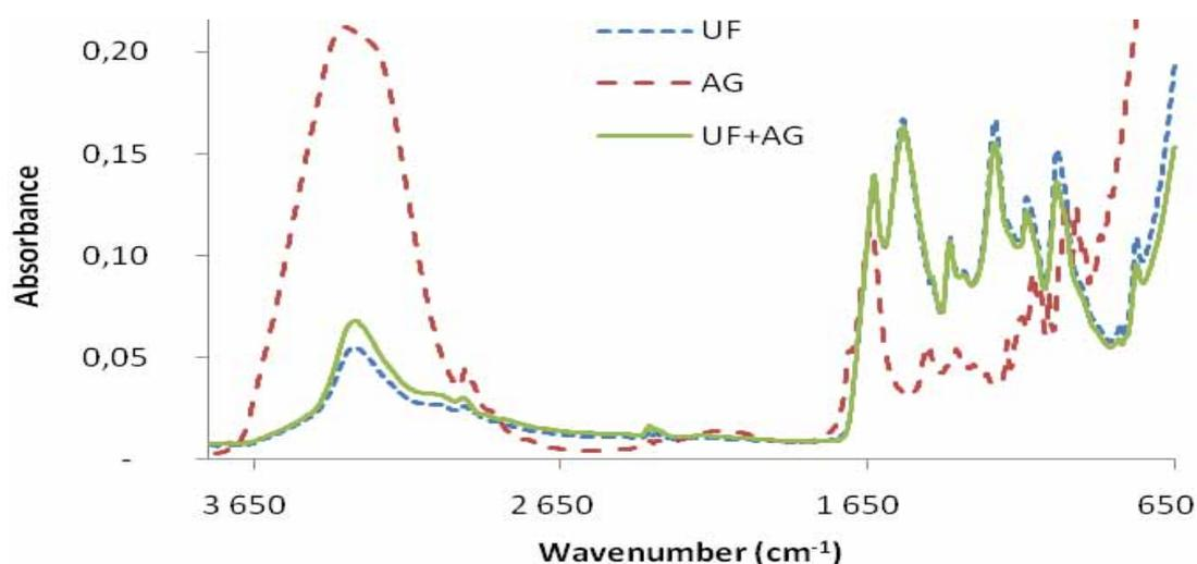
**Fig 3** FTIR spectra of UF adhesive and UF adhesive with GA
