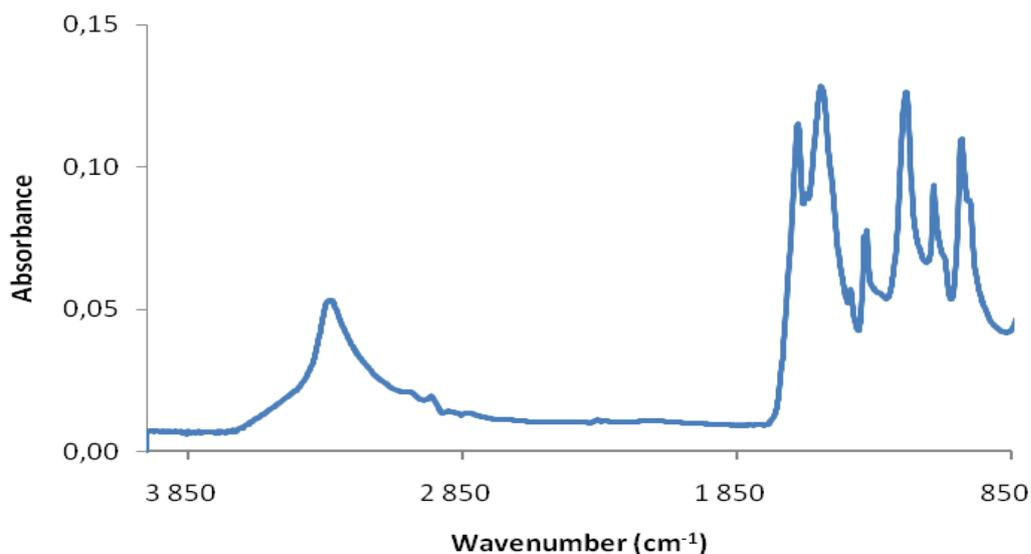
*Fig 4* FTIR spectra of UF adhesive and UF adhesive with GA and HK
