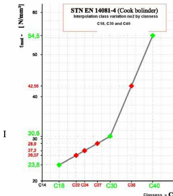
Fig. 2 Interpolation and extension of resistance class variation n°2 by classes C22, C24, C27 a C35.
