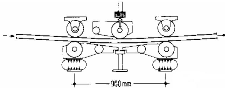
Fig. 1 Cook Bolinders SG-AF - scheme of three-point bending load on sawn timber
