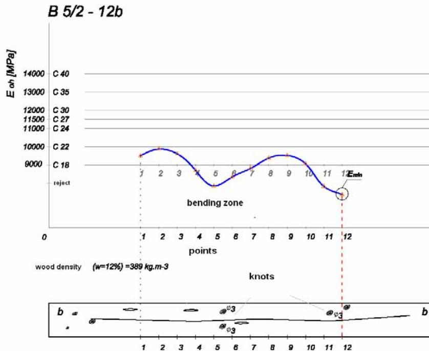
Fig. 4 Fluctuation of bending modulus of elasticity along the board B5/2 – 12p.
