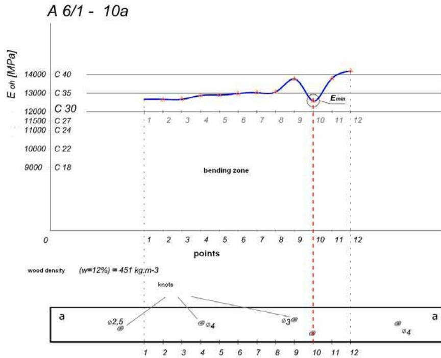
Fig. 3 The fluctuation of bending modulus of elasticity along board A 6/1
