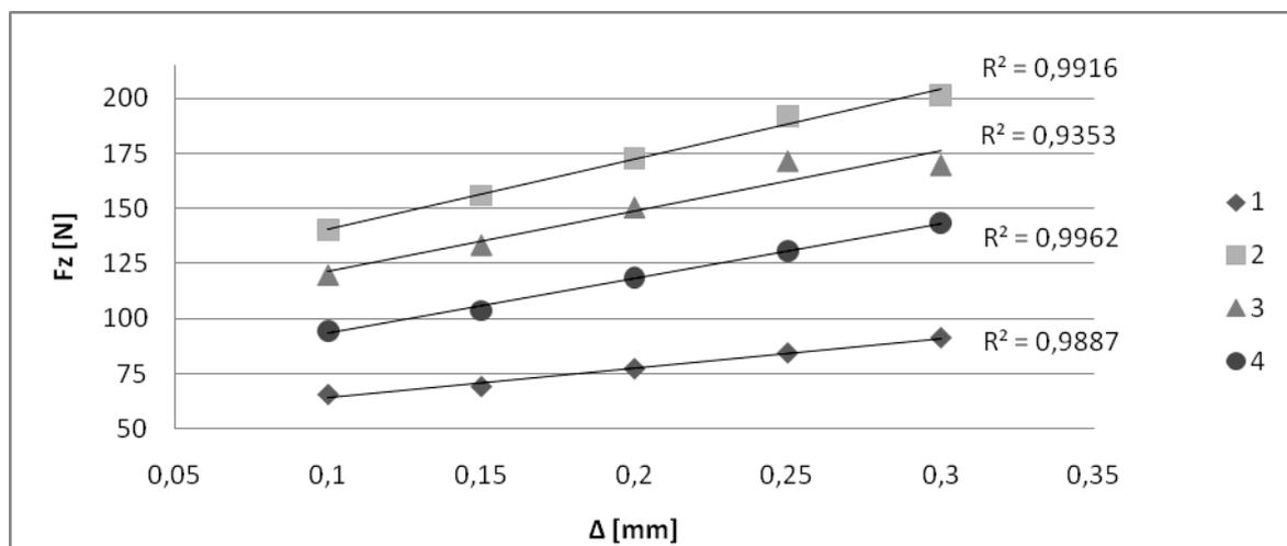
Fig. 4. Relationship between feed per revolution ( $\Delta$ ) and feed force ( $F_z$ ) for all tested materials (1- raw MDF, 2- raw particleboard, 3- laminated particleboard , 4- shuttering plywood)
