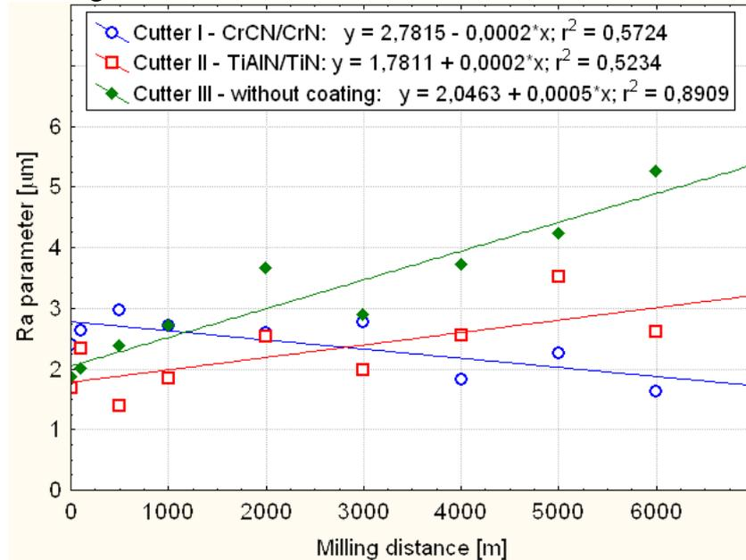
Fig. 3. Dependence of the arithmetic mean height Ra of the profile in the function of the milling distance for the examined cutters
