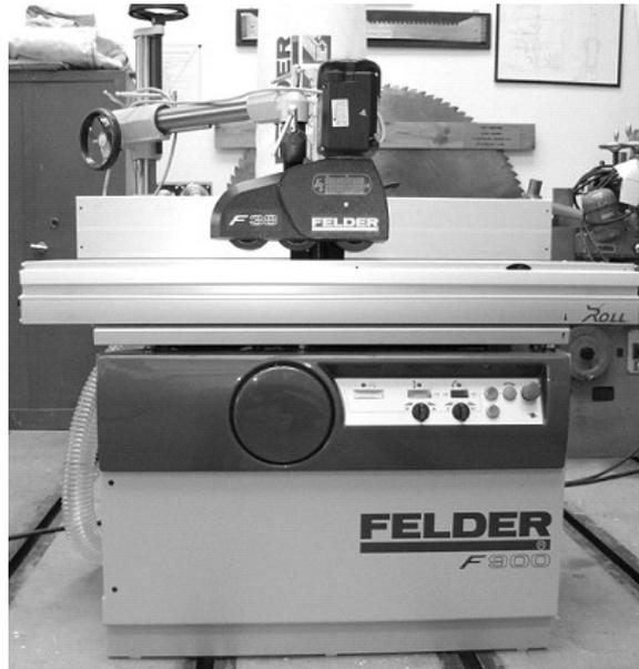
Fig. 1. Test stand of the bottom-spindle milling machine
