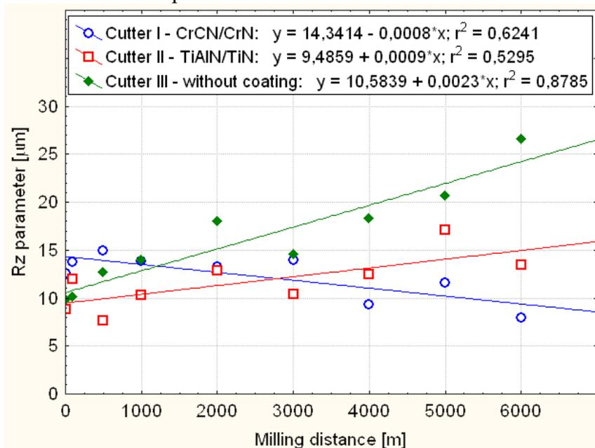
Fig. 4. Dependence of the average peak to valley roughness Rz in the function of the milling distance for the examined cutters
