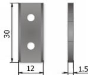
Fig. 2. Two-edge cutter blade used in experiments
