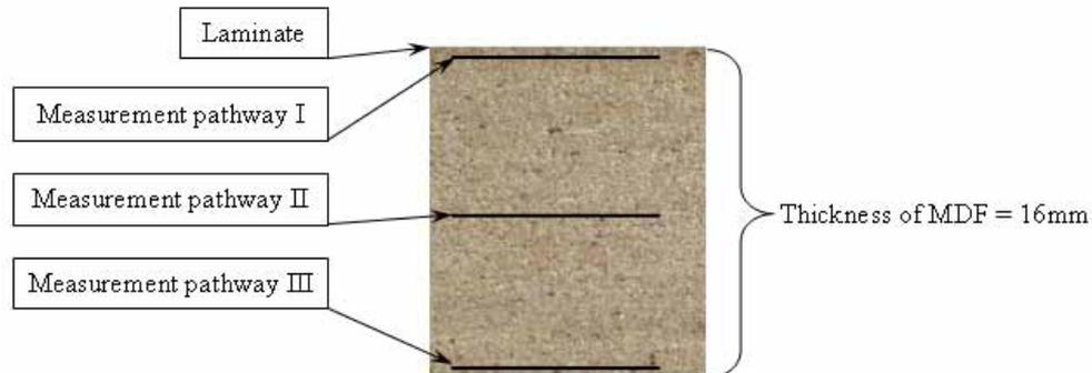
Fig. 1. Distribution of measuring pathways on the MDF
