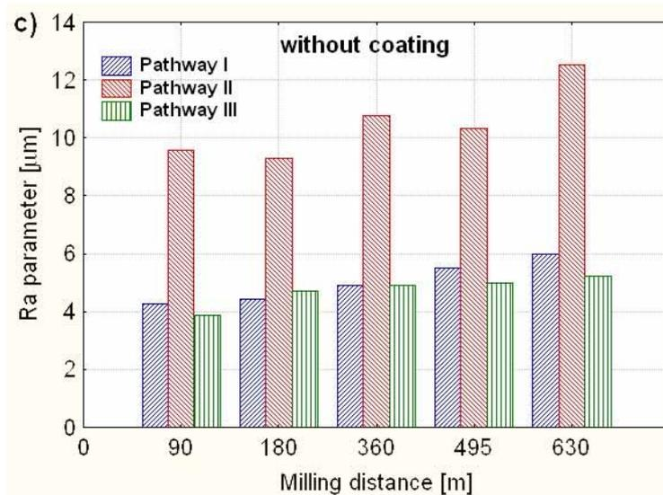
Fig. 4. Relationship between Ra parameter and machining distance for three measuring pathways for cutter edges: a) with CrCN/CrN coating, b) with TiAlN/TiN coating, c) without a coating
