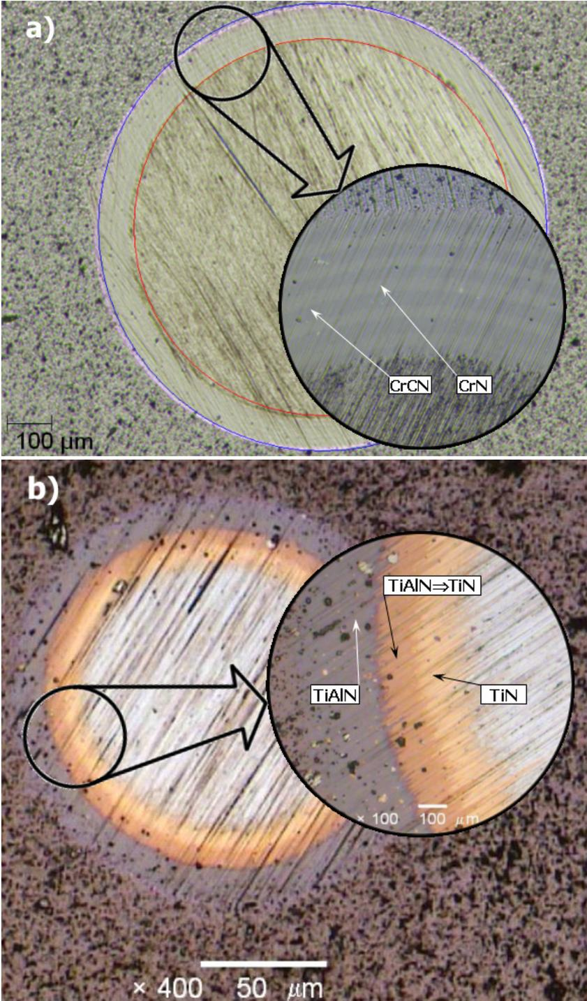
Fig. 3. Calotest friction track of the coatings: a) CrCN/CrN, b) TiAlN/TiN
