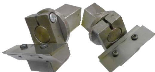
Fig. 2 Tool with skew cutting edge
