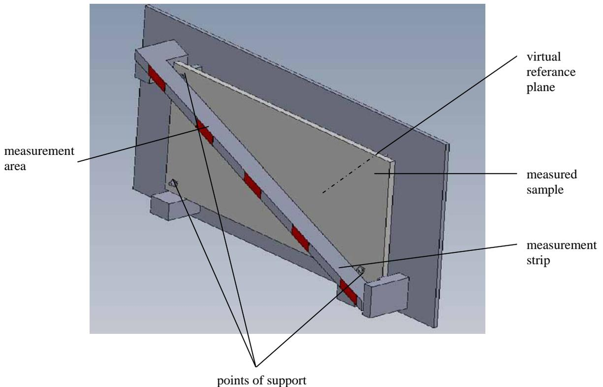
Fig. 1- Measurement stand with sample
