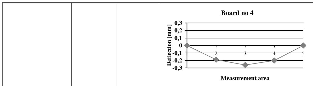
Obtain results show that it is no deformation of asymmetrical veneered wood-based boards after process of varnishing. The most deformed sample after varnishing was warped to 0,25mm in critical point (it was board veneered with European white birch and African Pterygota). It is also noticed that samples veneered with using hardwoods with higher porosity difference were more deflected than samples with lower porosity difference.
