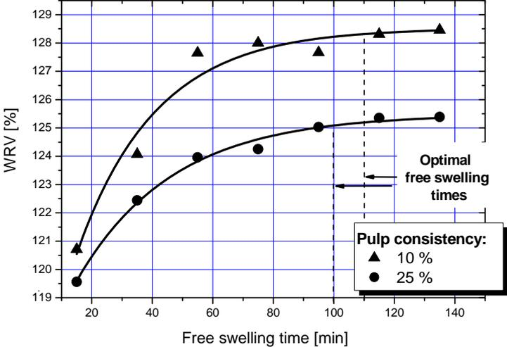
Fig. 2. Example of changes of water retention value (WRV) during free swelling of unbleached Kraft pine pulp previously refined in laboratory PFI mill (time of refining - 1 minute)
