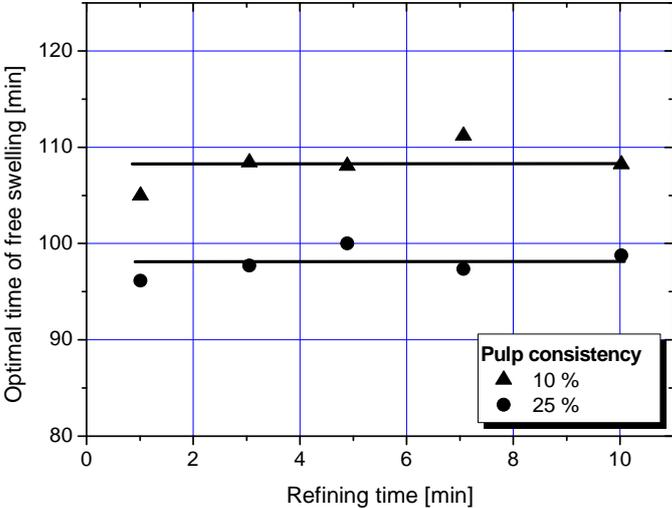
Fig. 3. Determination of optimum duration of free swelling for tested pulp refined under different refining conditions (time of refining)
