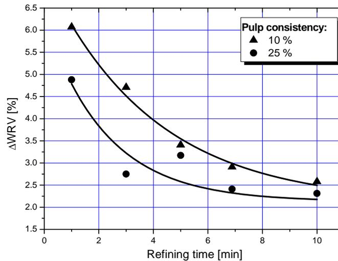
Fig. 4. Change of refined pulp WRV for different refining conditions
