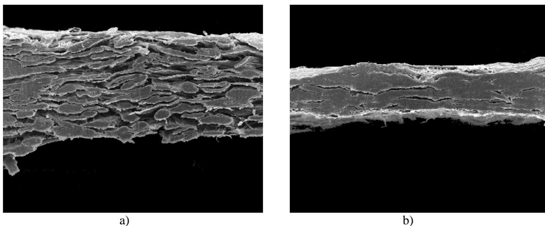
Fig. 1. a) Structure of paper made from unrefined pulp, b) Structure of paper made from refined pulp (flexible fibres). SEM photography, magnification x200
