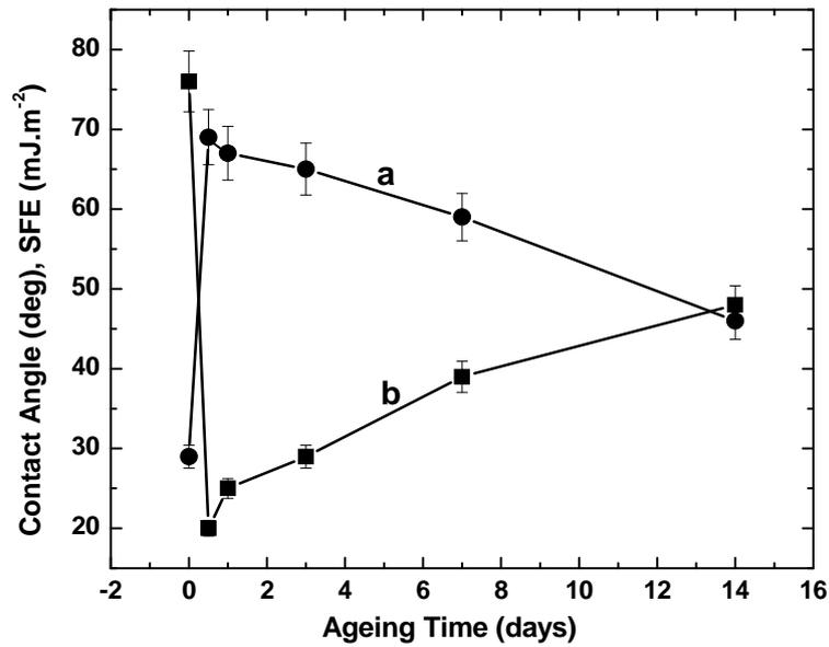
Figure 3. Surface energy (plot a) and contact angle (plot b) of oak wood surface modified by DCSBD plasma in oxygen vs. ageing time
