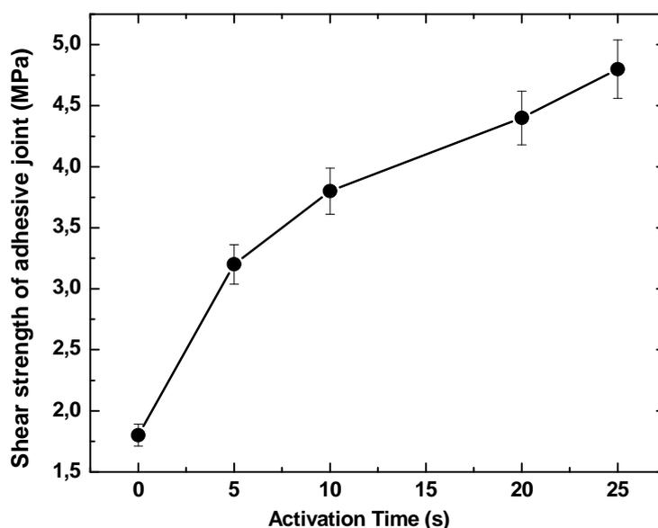
Figure 4. Shear strength of adhesive joint oak wood modified by DCSBD plasma in oxygen vs. activation time
