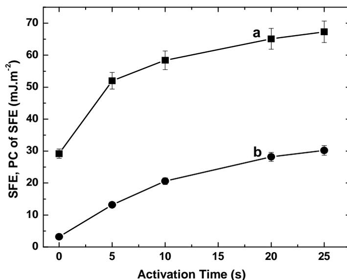
Figure 2. Surface energy (plot a) and its polar component (b) of oak wood modified by DCSBD plasma in oxygen vs. activation time
