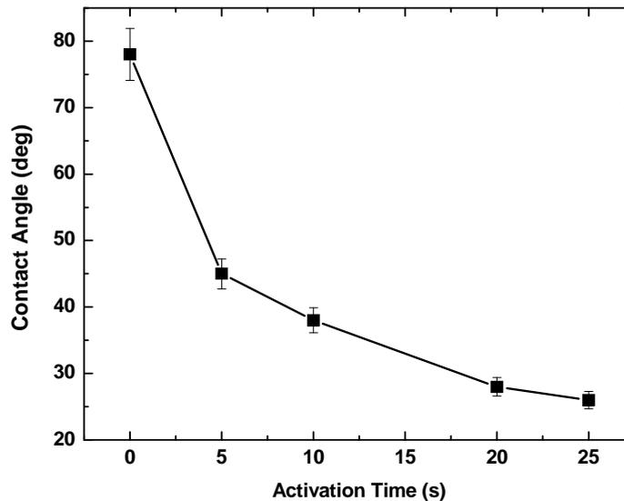
Figure 1. Contact angle of water deposited on oak wood surface modified by DCSBD plasma on oxygen vs. activation time
