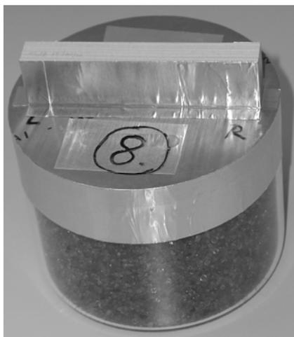
Fig. 1. Cup with silica gel and the sample above, isolated on four sides with aluminium tape
