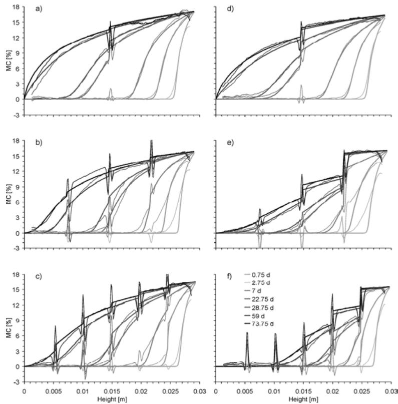
Fig. 2. Vertical profiles of the MC through the samples with 1, 3 and 5 adhesive joints of series 1 during the diffusion experiment (experimental results = fine lines; model curves = fat lines):
