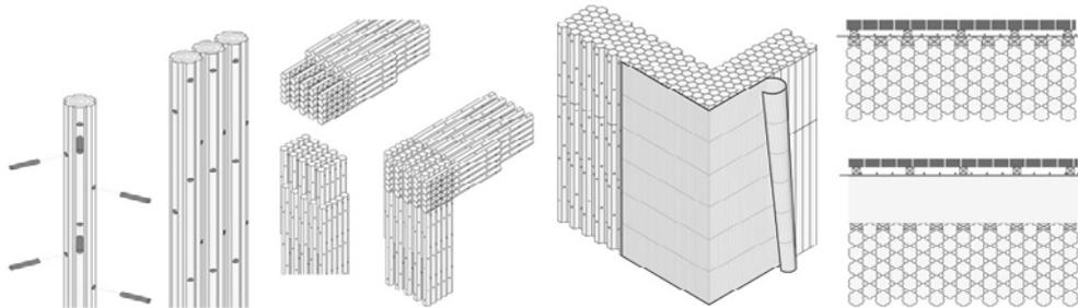
Picture. 3 Construction elements in Palisadio system
