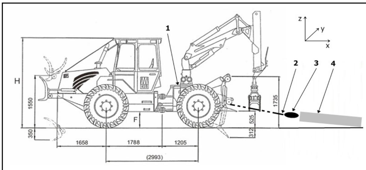
Fig. 1. Schema of the work by the skidding
