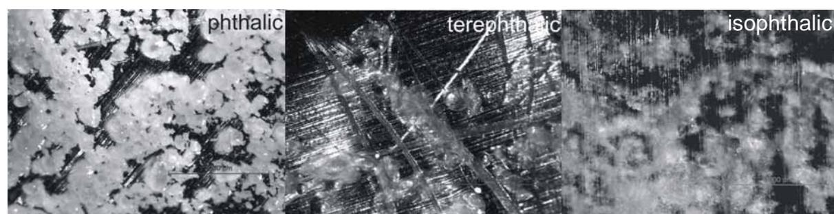
Fig. 4 Microphotographs of the polyesters of aromatic dicarboxylic acids
