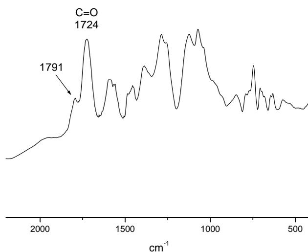
Fig. 3 FTIR spectrum of polyester from HBP-1W and phthalic anhydride cured at  $170^{\circ}\text{C}$  for 15 min in the presence of imidazole as a catalyst
