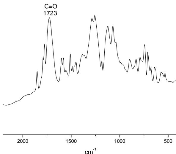
Fig. 4 FTIR spectrum of polyester Bis101 and phthalic anhydride cured at 170°C for 15 min in the presence of imidazole as a catalyst
