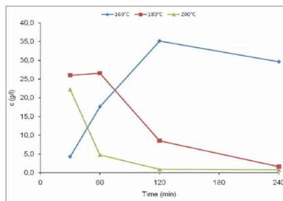
**Fig. 2** Influence of temperature and reaction time on the concentration of released mono- and oligosaccharides from ash wood.
