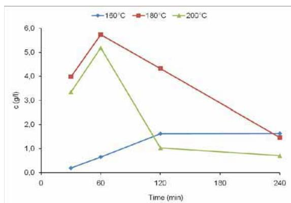
**Fig. 1** Influence of temperature and reaction time on the concentrations of released monosaccharides from ash wood.
