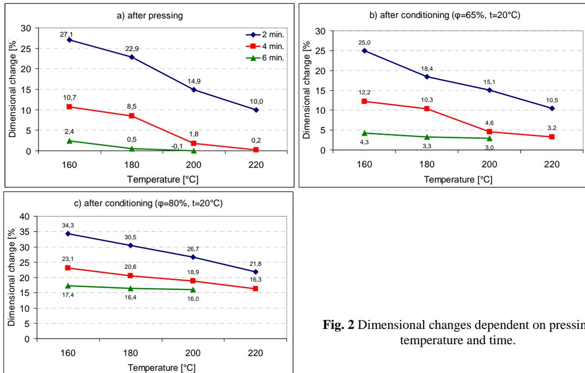
**Fig. 2** Dimensional changes dependent on pressing temperature and time.
