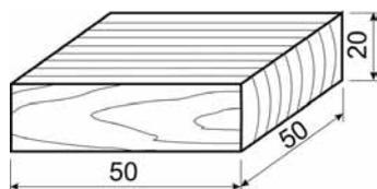
**Fig. 1** Dimensions and shape of test specimens
