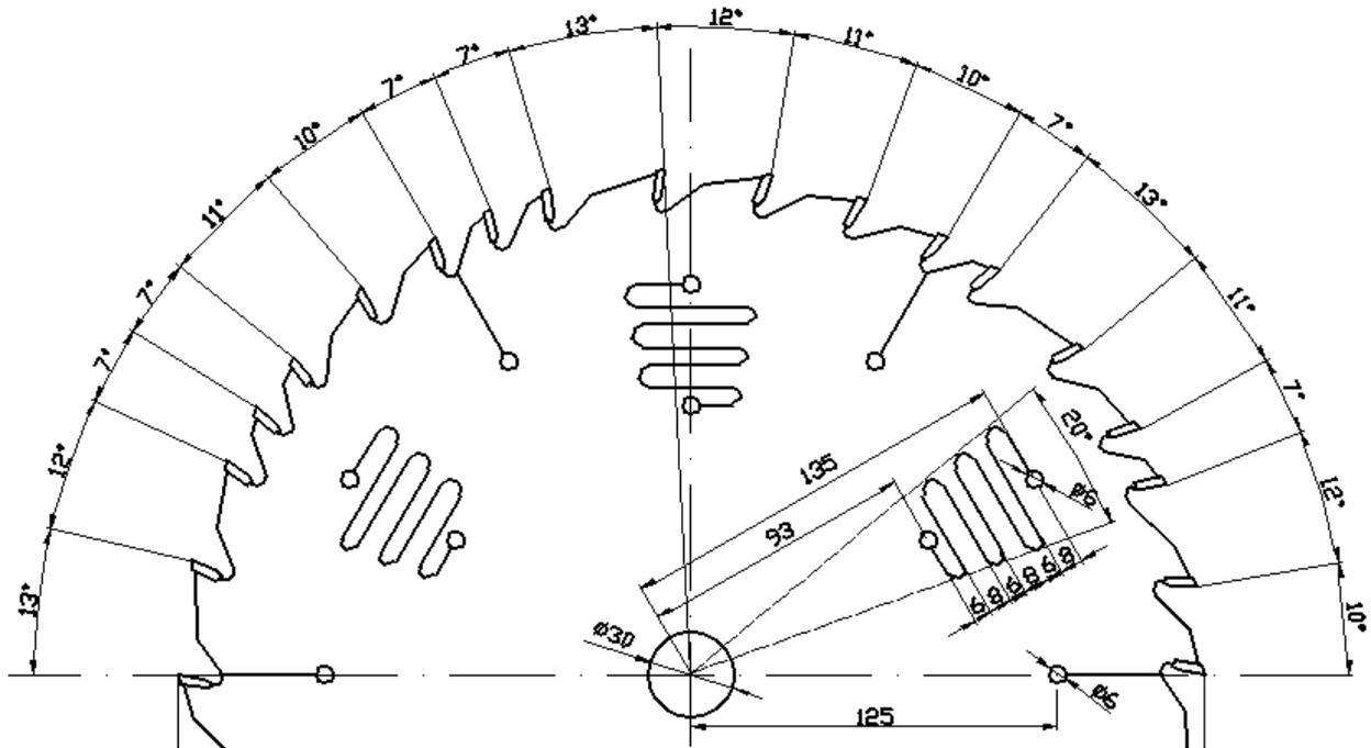
Fig. 3 Tested circular-saw blade – K8
