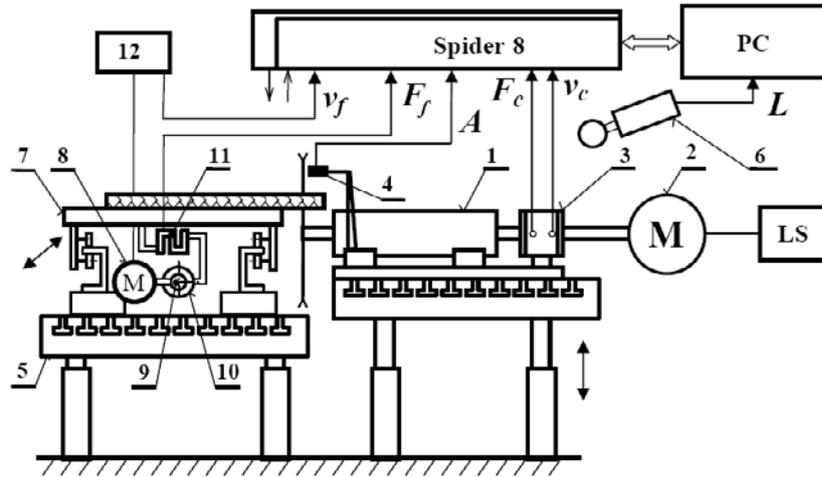
1 – spindle, 2 – electric motor with rpm regulation LS, 3 - cutting force  $F_c$  and speed  $v_c$  sensor, 4 – contactless sensor of vibrations  $A$ , 5 - grate table, 6 - noise meter, 7 – feeding carriage, 8 – electric motor for the carriage feed, 9 - ball screw, 10 – nut, 11 – feeding force sensor  $F_f$ , 12 – frequency converter for the feeding speed change  $v_f$
