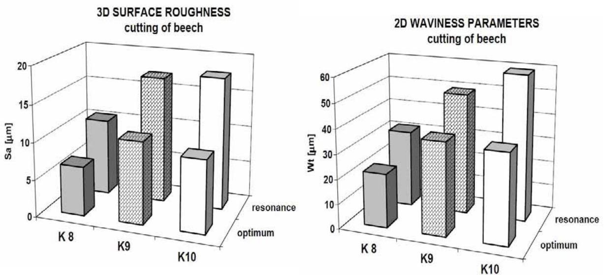
Fig. 9 Comparison of the surface roughness and waviness at cutting beech by disks K8, K9, K10
