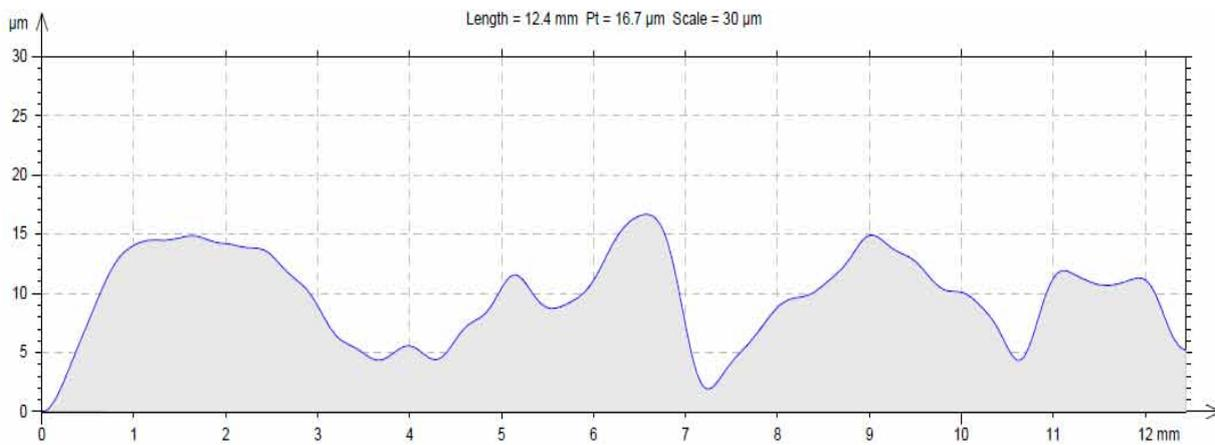
Fig. 8 Waviness – cutting by a disk K8,  $n_{opt} = 4100 \text{ min}^{-1}$
