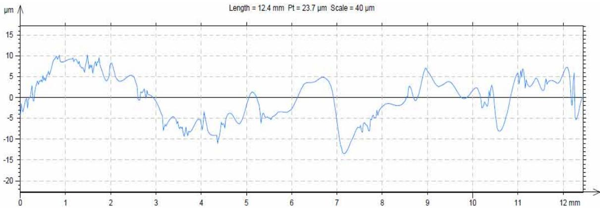
Fig. 7 2D cut of a profile from the basic area – cutting by a disk K8,  $n_{opt} = 4100 \text{ min}^{-1}$
