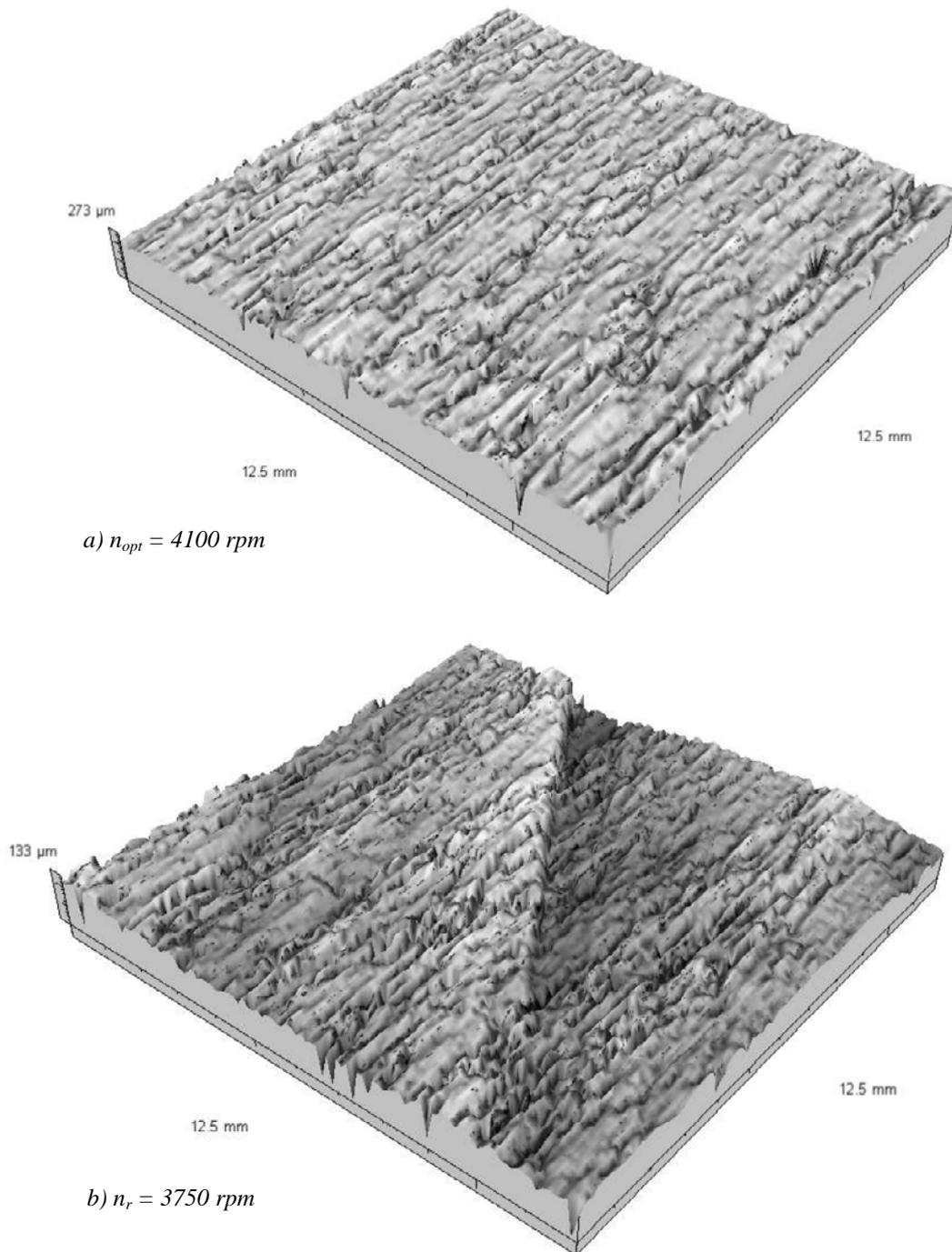
Fig. 6 3D basic profile of the surface – beech, K8
