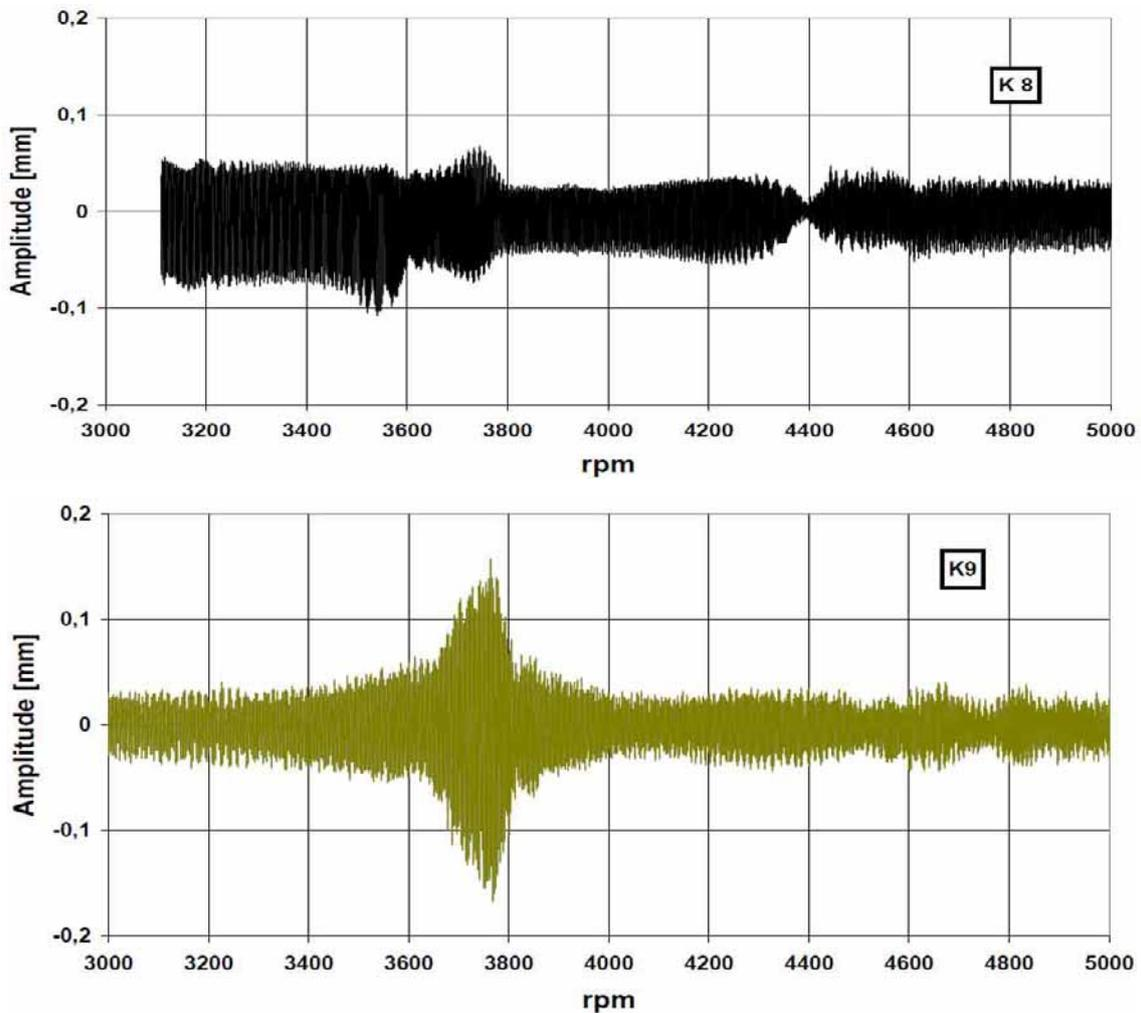
Fig. 4 The course of vibrations of circular-saw blades
