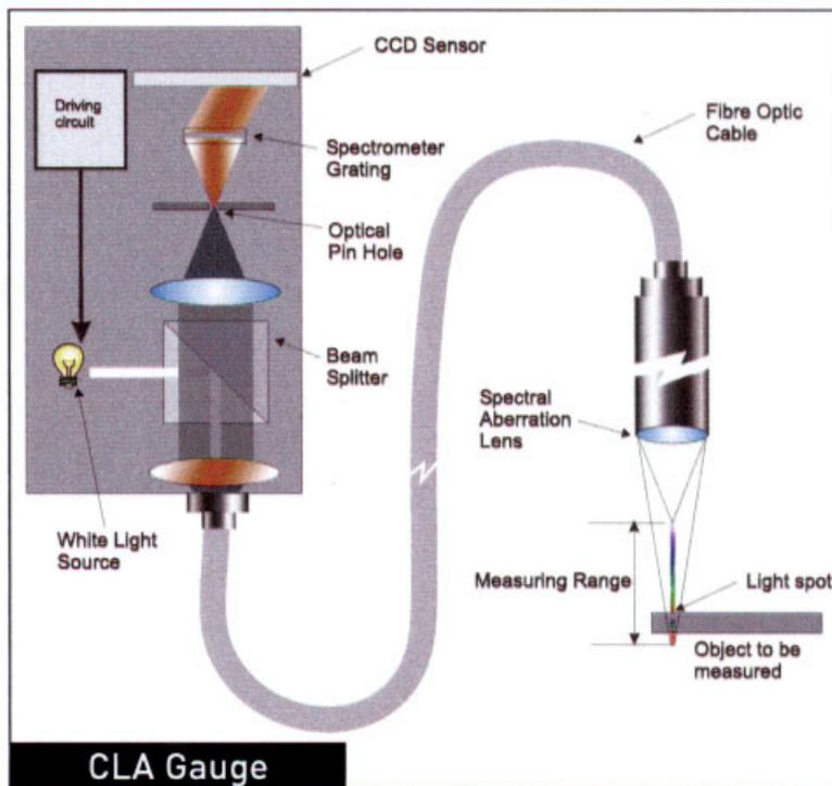
Fig. 2 Confocal sensor CLA
