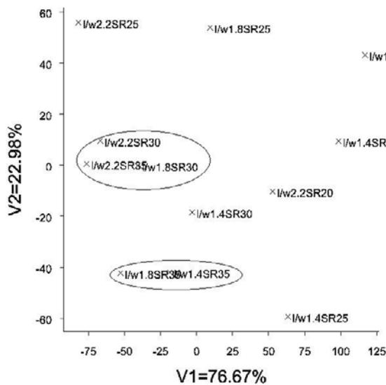
The first group of higher l/w and freeness and the second one of lower l/w and the highest freeness do not differ significantly the pulp strength properties. The rest of the l/w and SR freeness pairs, especially pulp refined to 20°SR and 25°SR have differed strongly the mechanical factors. It can be explained by well known phenomenon: the increase of 5°SR freeness at the beginning brings more fiber strength than at the end of refining [Markstrom 1995].
