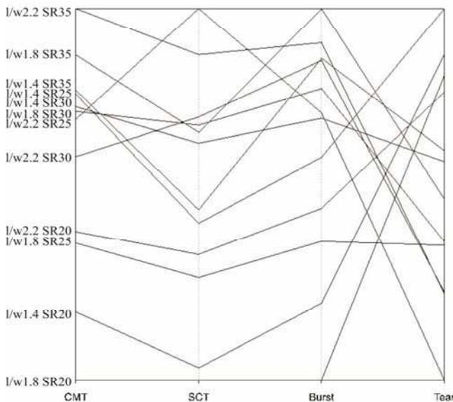
The lines close to parallel and with similar angle of inclination have been marked as “positive”. Nine positive correlations between CMT and SCT for all tested l/w ratio and freeness can be distinguished. The best results (CMT, SCT, Burst) were achieved for combination of variables 2.2 l/w and 35°SR. However two data sets for 2.2 l/w have shown negative correlation with middle freeness: 25°SR and 30°SR.
