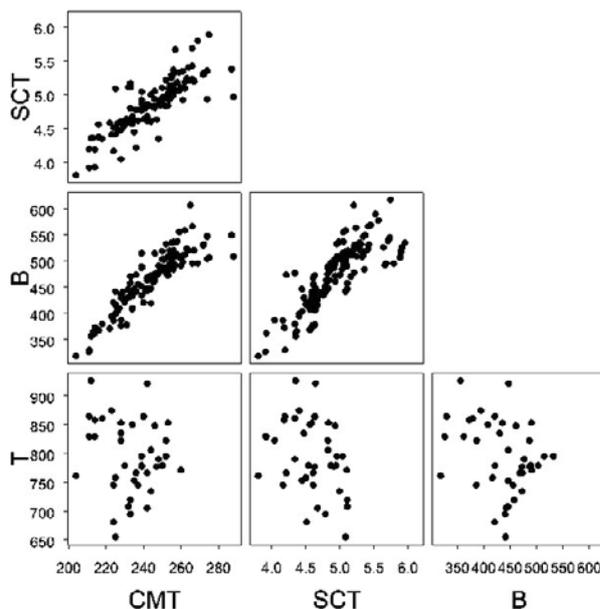
Fig. 1 Scatter plot of CMT, SCT, Burst (B) and Tear (T) strength correlation.
