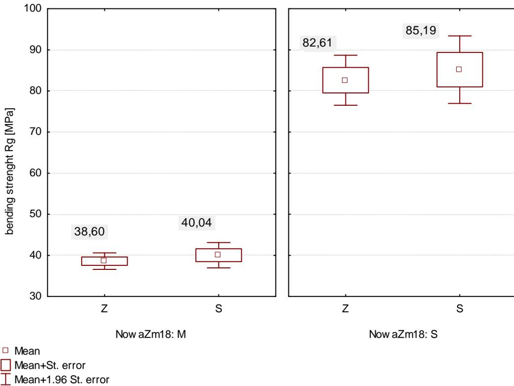
Fig. 3 Static bending strength ( $R_g$ ) of wood with moisture content exceeding the fiber saturation point (M) and absolutely dry wood (S)
