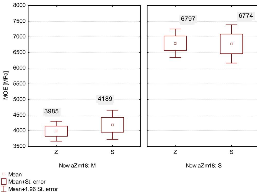
Fig. 4 Modulus of elasticity at static bending in wood with moisture content exceeding fiber saturation point (M) and absolutely dry wood (S)
