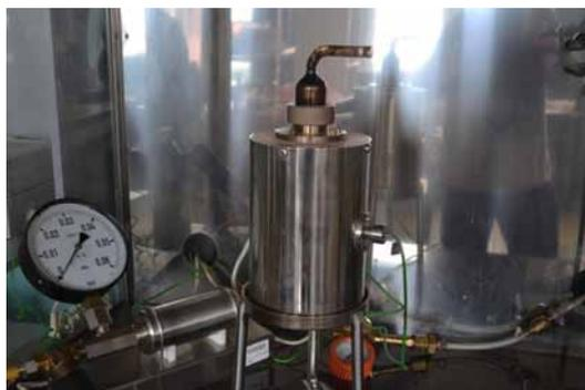
Fig.2. The test stand for determining the ignition temperature of cloud of dust
