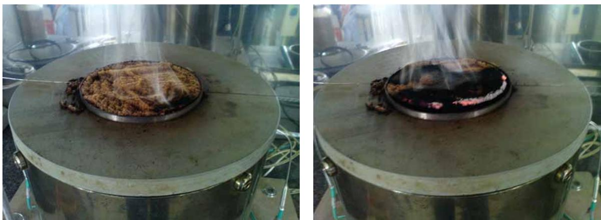
Fig.3. Emission of smoke from wood dust during the measurement: a) initial phase, b) final phase
