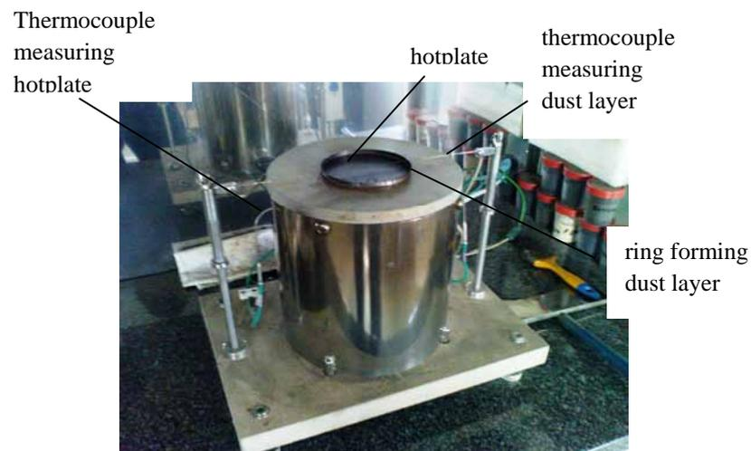
Fig.1. The test stand for determining the ignition temperature of layer of dust
