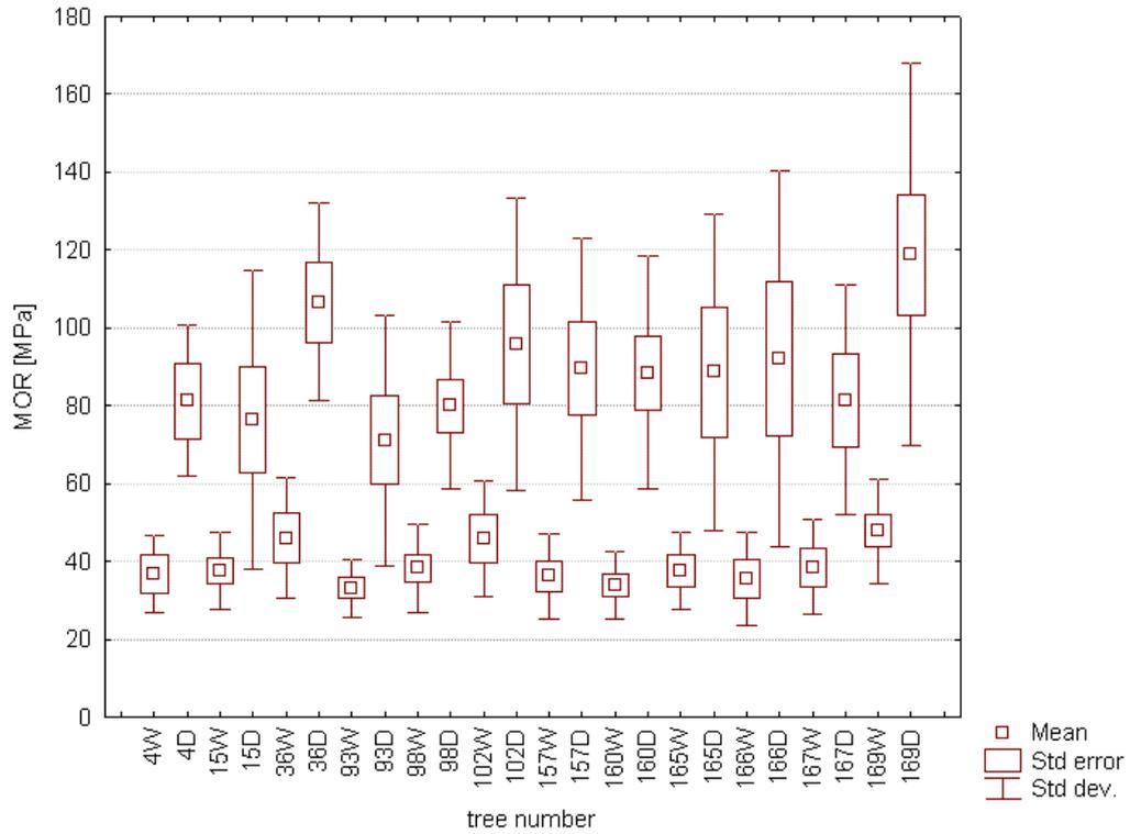
Fig. 1 A comparison of static bending strength of trees in samples tested at a moisture content above fiber saturation point (W) and absolutely dry samples (D), Świdwin.
