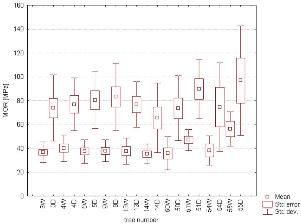
Fig. 2 A comparison of static bending strength of trees in samples tested at a moisture content above fiber saturation point (W) and absolutely dry samples (D), Kolbody.
