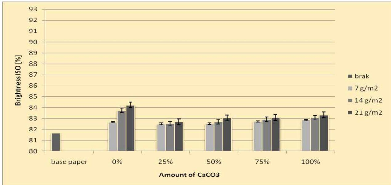
Figure 2: Effect of calcium carbonate content in kaolin and carbonate coating on paper ISO brightness
