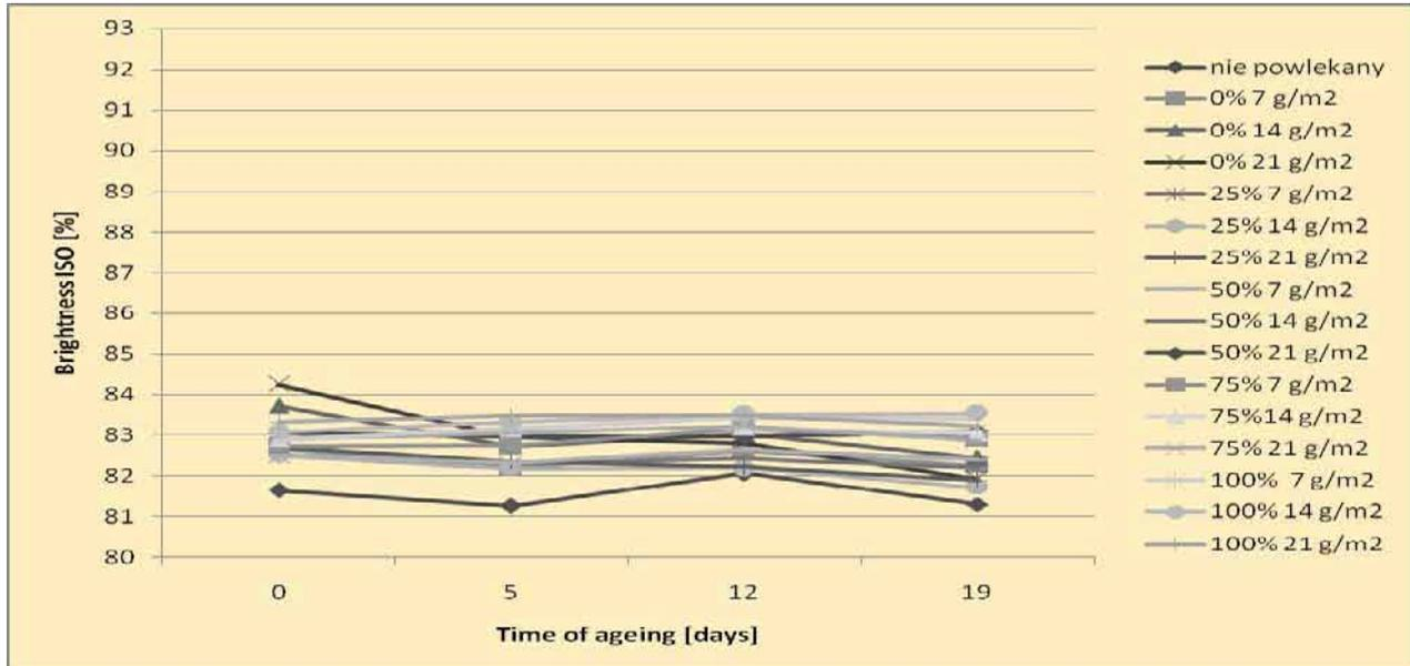
Figure 4: Effect of ageing time with outdoor daylight in closed room on ISO brightness of paper with kaolin and calcium carbonate coatings
