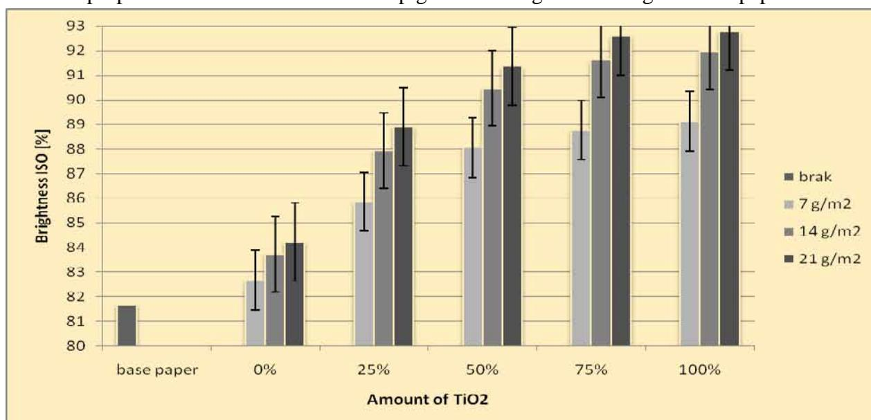
Figure 1: Effect of titanium dioxide amount in kaolin and rutile coating on ISO brightness
