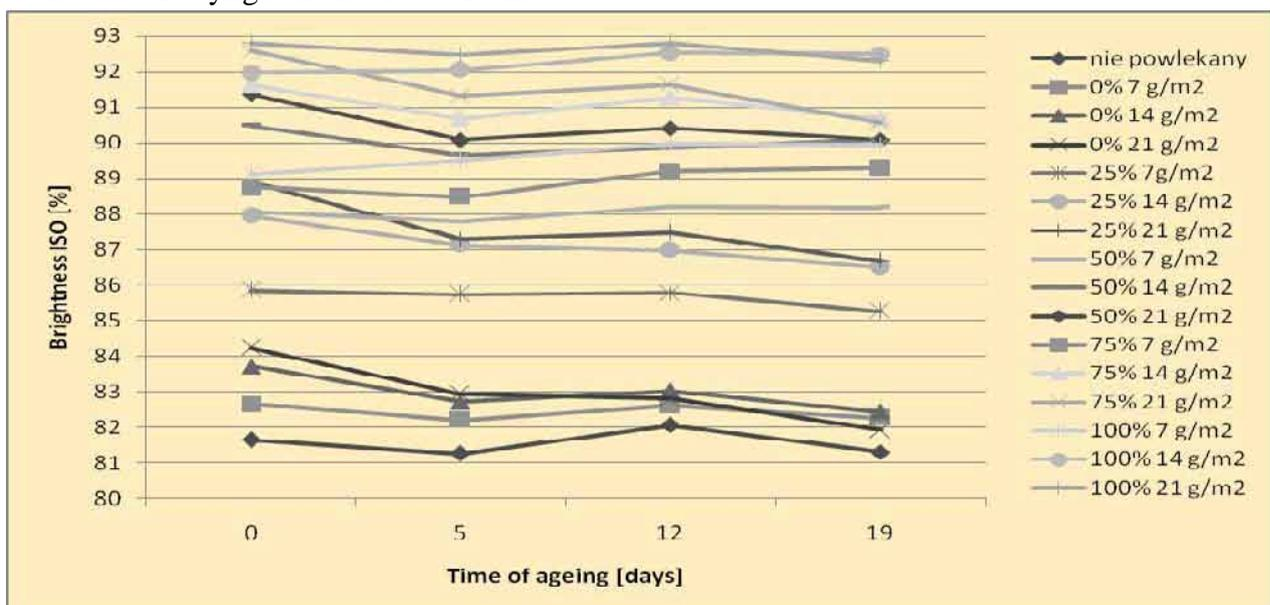
Figure 3: Effect of ageing time with outdoor daylight in closed room on ISO brightness of paper with kaolin and rutile coatings
