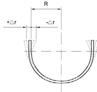
Fig. 2 Schematic description of deforming (closing, opening) of laminated part shaped in “U”
