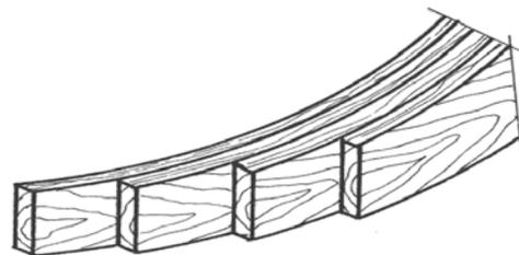
Fig. 1 Arrangement of lamellas in laminated wood
