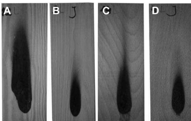
Fig. 1. Samples after test of reaction to fire: A - unprotected pine slat, B - impregnated pine slat, C – unprotected beech slat, D - impregnated beech slat.
