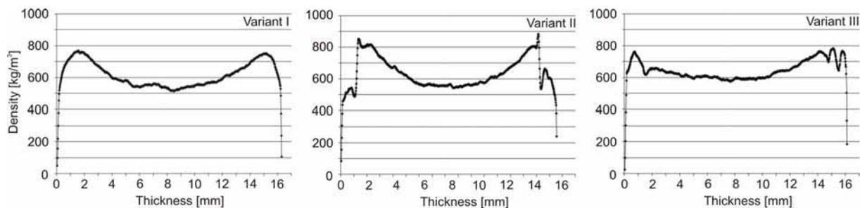
Fig. 1. Density distribution of tested boards
