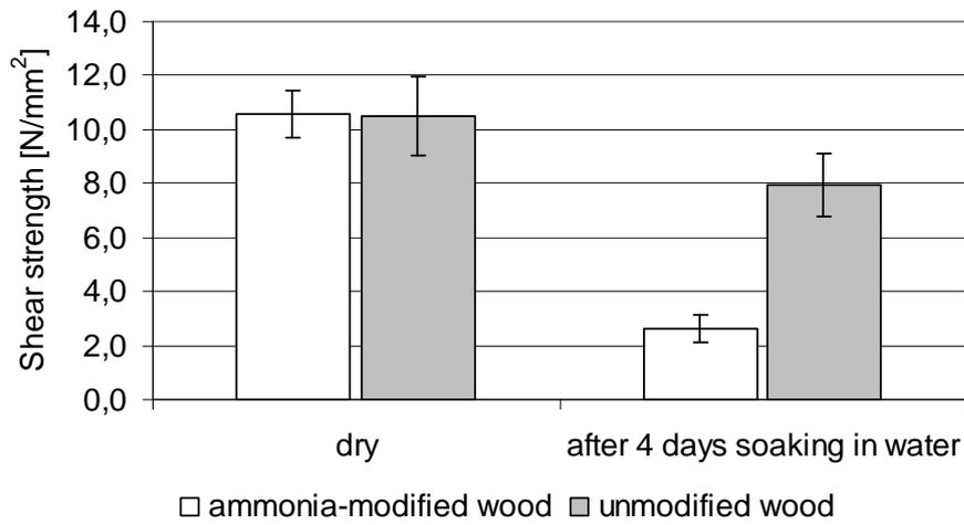
Fig. 1. Shear strength results of Black locust samples glued with MUF.
