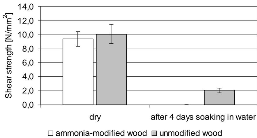
Fig. 2. Shear strength results of Black locust samples glued with PVAc
