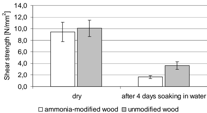
Fig. 3. Shear strength results of Black locust samples glued with EPI
