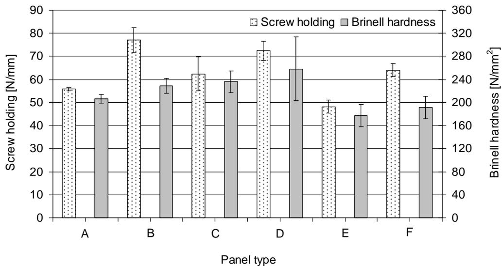
Fig. 2. Screw holding ability and hardness of the boards
