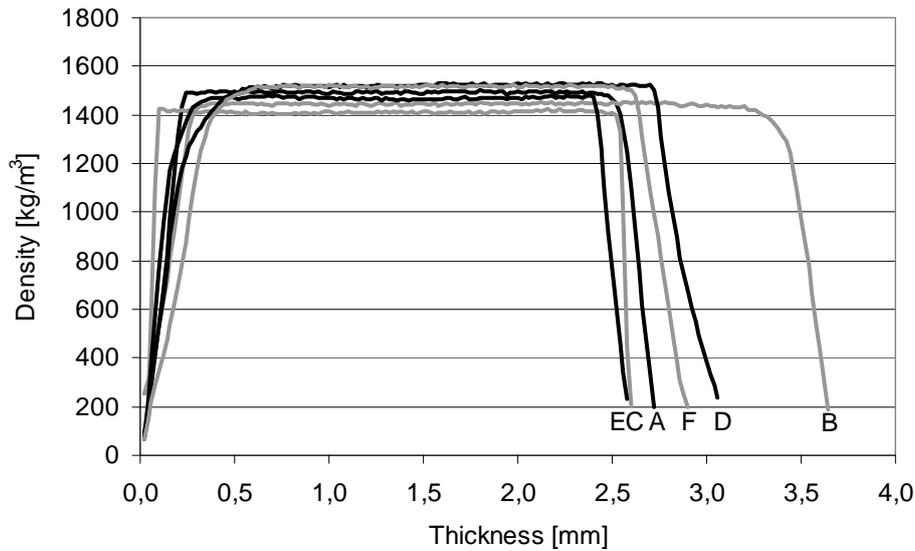
Fig. 1. Cross-sectional density profiles of the tested boards
