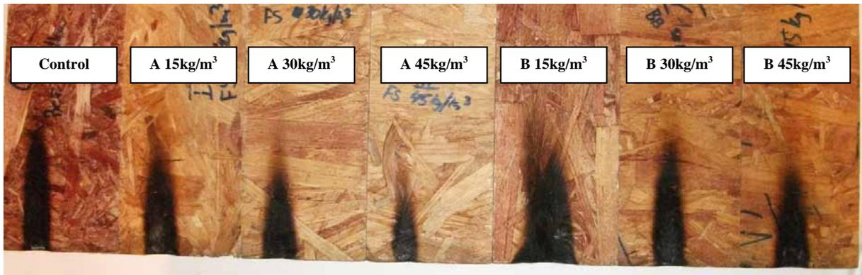
Fig. 1. Samples after single-flame source test – test was conducted on the basis of oxygen index method.
