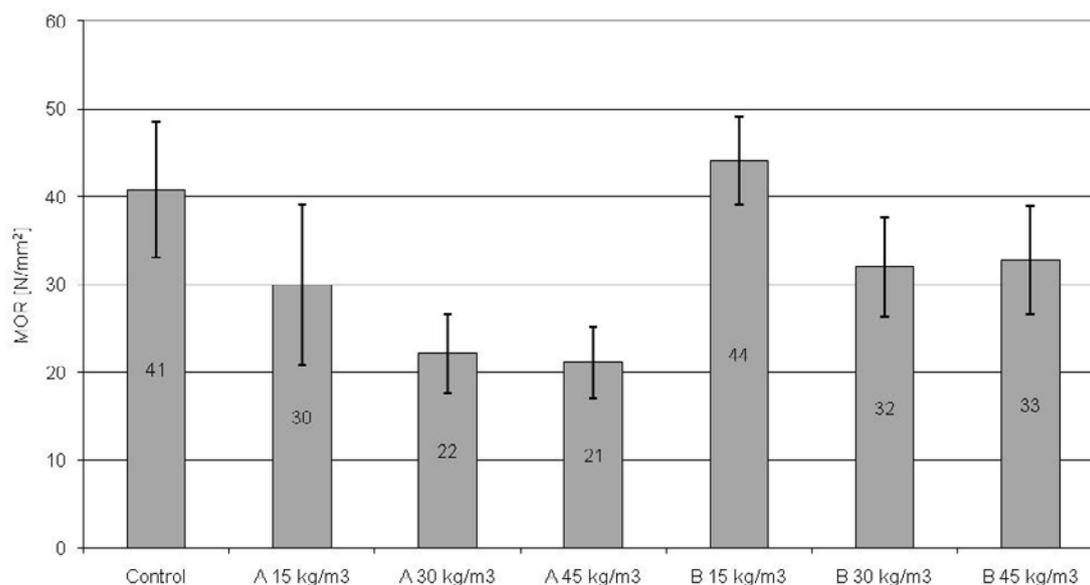
Fig. 3. Static bending strength (MOR) for particular variants.
