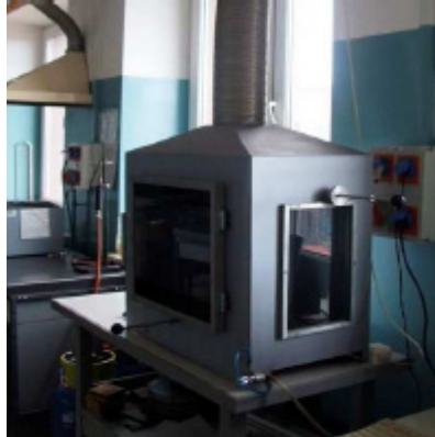
Fig. 2. Stand for flammability test of materials treated with direct flame influence, according to PN-EN ISO 11925-2:2004 in laboratory of Department of Combustion and Fire Theory, The Main School of Fire Service – SGSP
