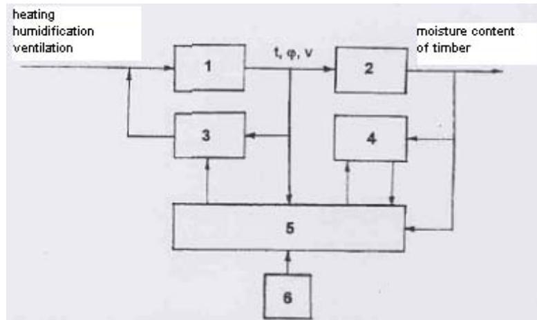
Fig. 2. Block scheme of control system of the dryer with the use of expert system: 1 - dryer chamber. 2 - timber in the dryer, 3 - controller, 4 - computer, 5 - expert system, 6 - operator
