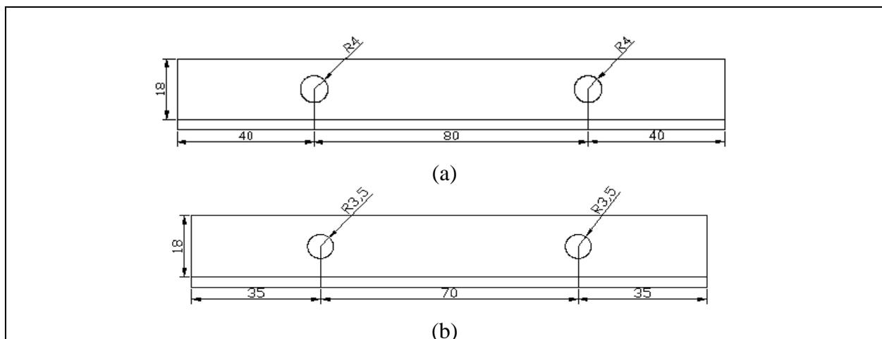
Figure 3. The distance between center of screw holes for bending (a) and tension (b) tests (in mm)
