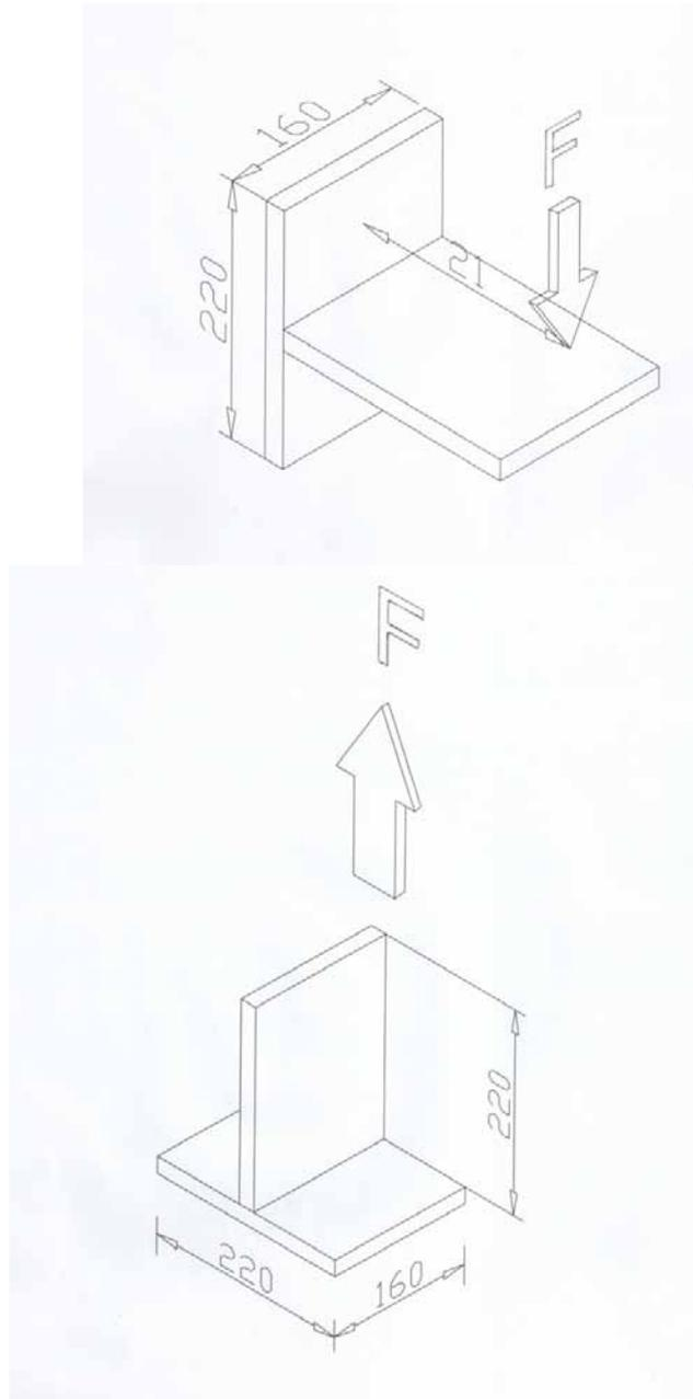
Figure 4. General configuration of the test setup used in the study for bending (a) and tension (b) tests (in mm)
