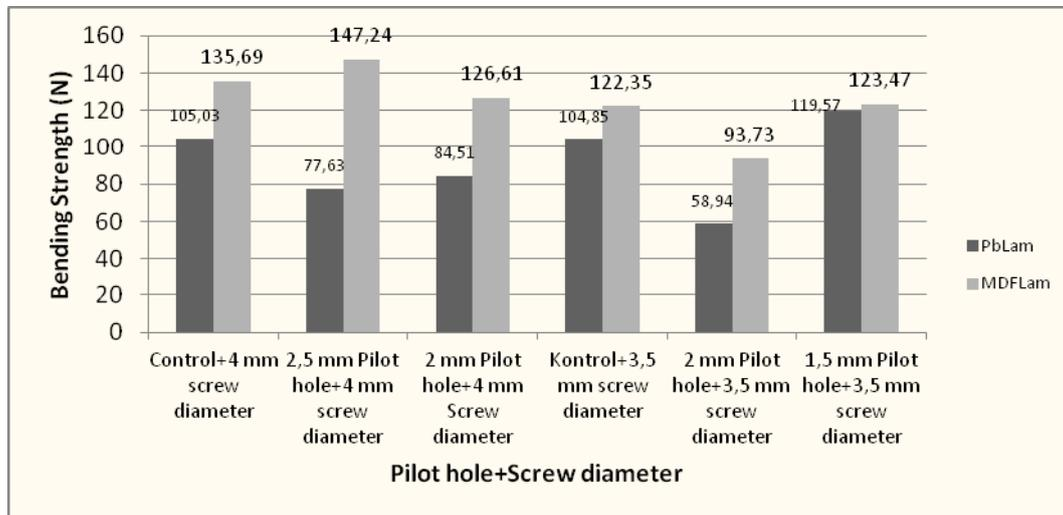
Figure 5. Effect of pilot hole and screw diameter on bending strength of T-type joints
