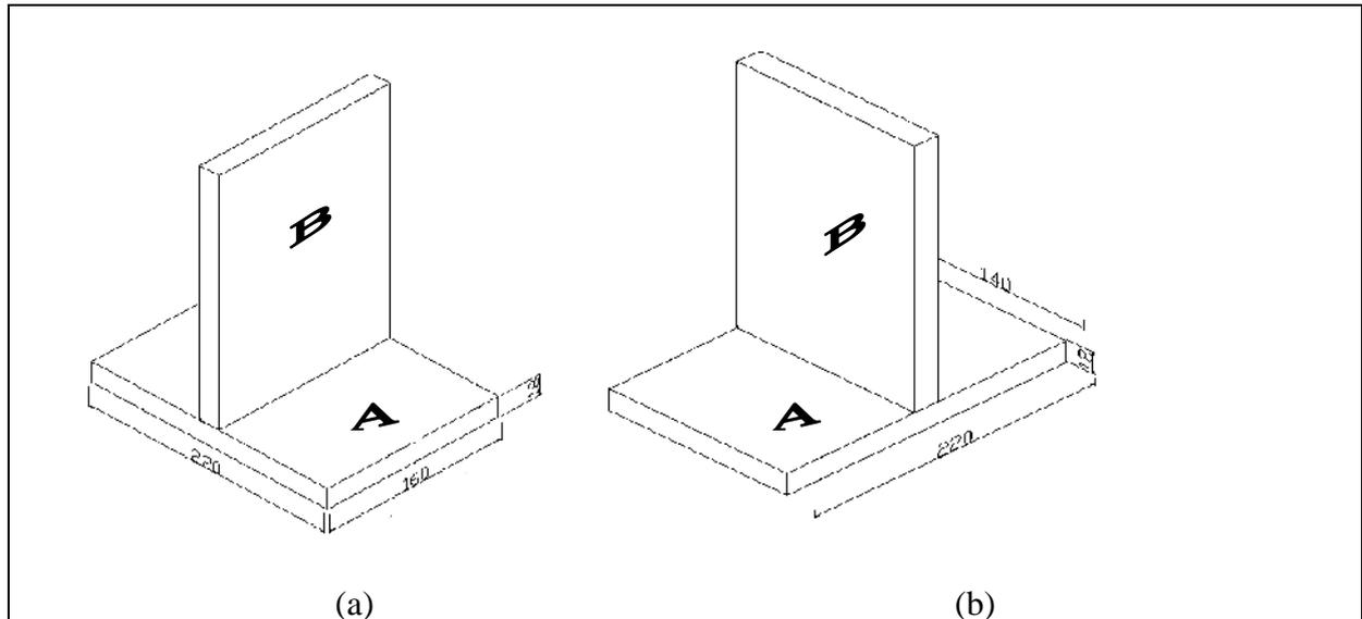
Figure 2. General configuration of the specimens for bending (a) and tension (b) tests in mm
