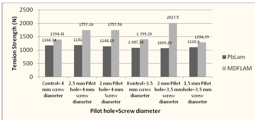
Figure 6. Effect of pilot hole and screw diameter on tension strength of T-type joints
