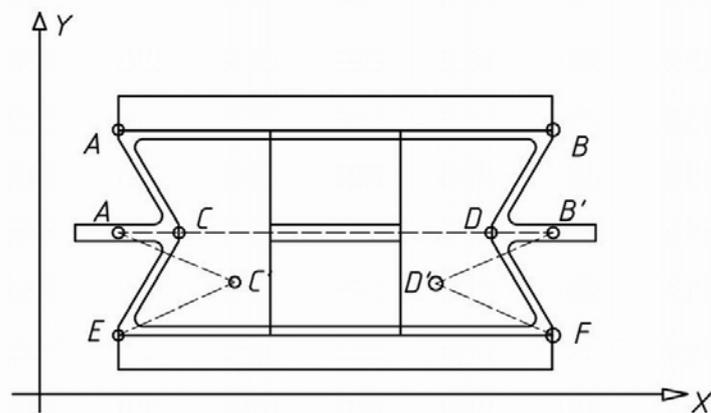
Figure 14. Sketch for calculation of spring Poisson ratio
