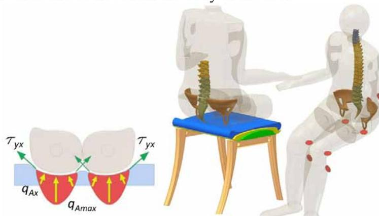
Figure 3. A diagram for the distribution of pressures and friction forces on the body of the user when sitting
