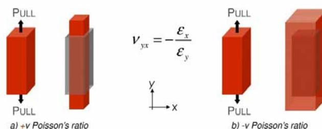
Figure 1. Uniaxial tension test of: a) conventional, and b) auxetic materials.
