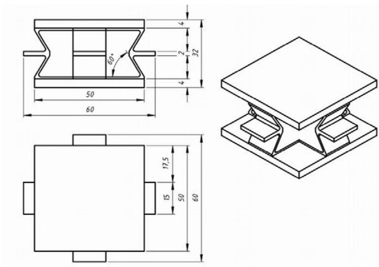
Figure 4. A model of a push spring with auxetic properties
