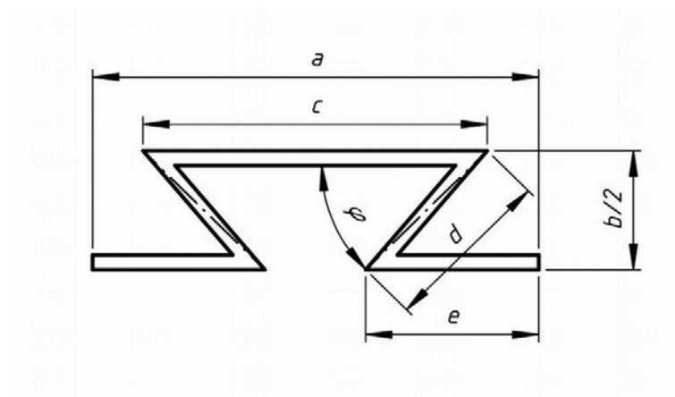
Figure 6. A computational model for the length of foot rockers
