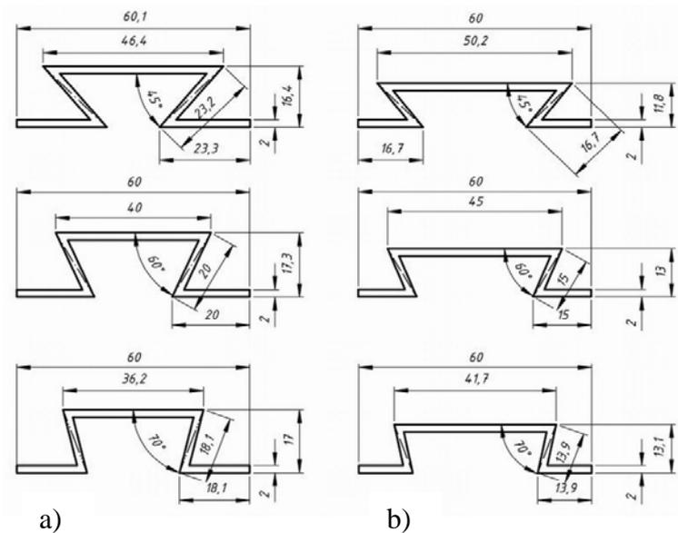
Figure 7. Examples of different foot geometries. a) tall and narrow, b) low and wide.
