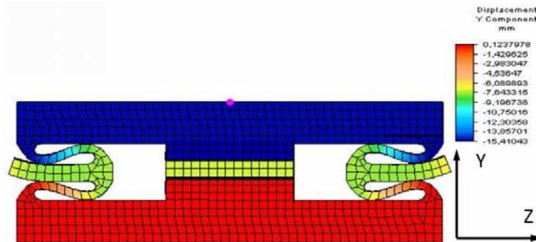
Figure 12. Deflection of a spring in the state of uniaxial compression
