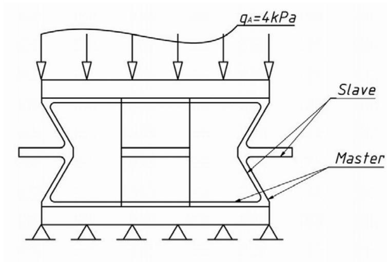
Figure 8. A diagram of loading for a single spring
