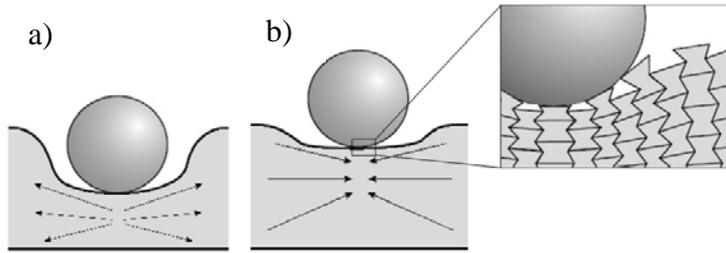
Figure 2. A diagram for the action of a rigid body on: a) conventional, and b) auxetic foundations.
