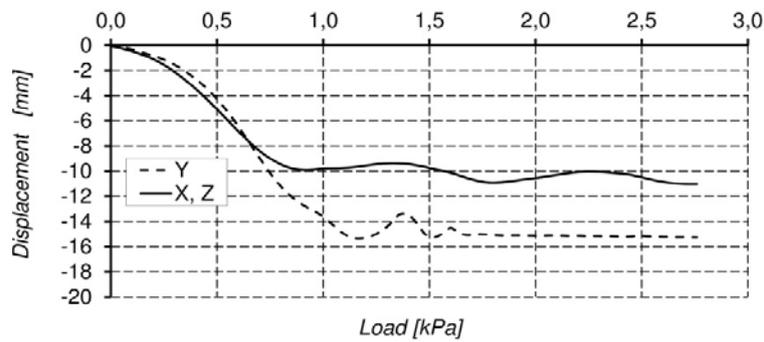
Figure 13. Deflection along the Y axis and displacements along the X, Z axes
