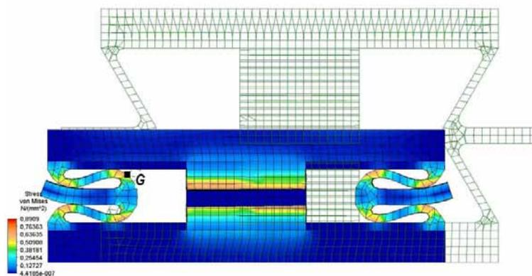
Figure 15. The distribution of von Mises reduced stresses
