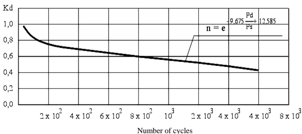
Figure 3 Relation between dynamic load coefficient and number of dynamic loads cycles according to Dziegielewski
