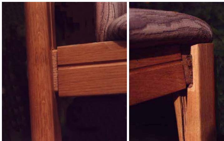
Figure 2 Pulling out and rupture caused by load
