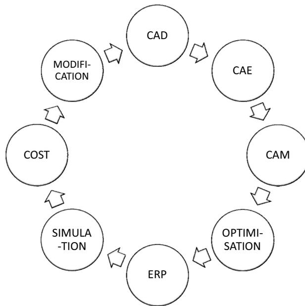
Figure 1. Proposed cycle of preparation and assessment of a design alternative with the use of numerical optimization
