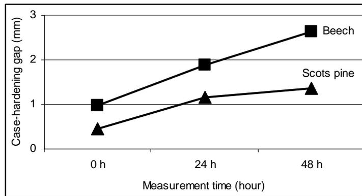
Figure 2. Casehardening gap values of vacuum dried wood samples
