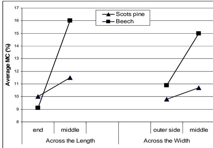
Figure 1. MC distribution across the length and width of the vacuum dried samples
