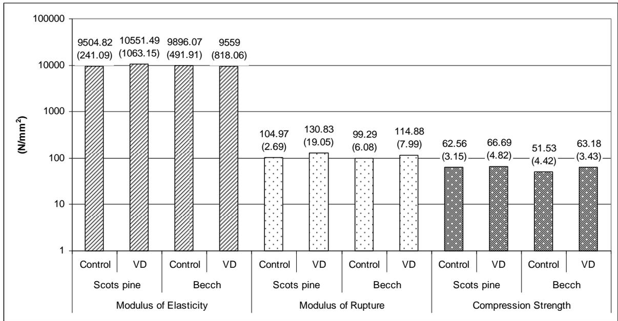
Figure 3. Mechanical properties of Scots pine and Beech wood (VD indicates Vacuum Drying and Values in the parenthesis indicate standard deviation)
