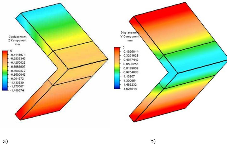
Fig. 9. Size of deflection: a)  $\delta_{1P}$  of the joint with the element of substitute rigidity ( $E_z^Z$ ) subjected to closing,  $\delta_{1P(\max)}=1.42$  mm, b)  $\delta_{2P}$  of the joint with the element of substitute rigidity ( $E_z^R$ ) subjected to opening,  $\delta_{2P(\max)}=1.62$  mm
