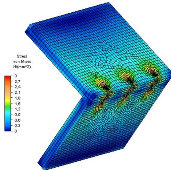
Fig. 4. Distribution of reduced stresses according to Mises in a dowel joint subjected to closing,  $\sigma_{\max} \approx 3 \text{ MPa}$
