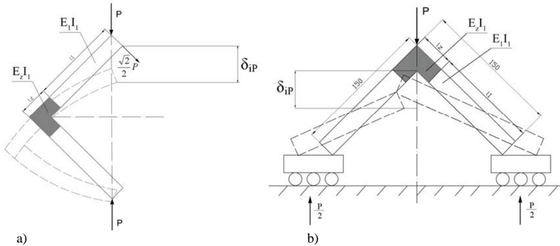
Fig. 2. Diagram of loading of the angle joint in: a) closing, b) opening tests
