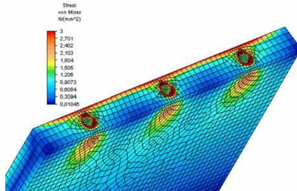
Fig. 6. Distribution of reduced strains according to Mises on the surface of seats in a dowel joint subjected to closing,  $\sigma_{\max} \approx 3$  MPa
