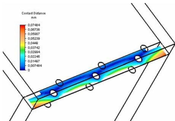
Fig. 7. Size of gap between boards pressing against each other in the joint subjected to closing,  $\delta_{\max} \approx 0,08$  mm
