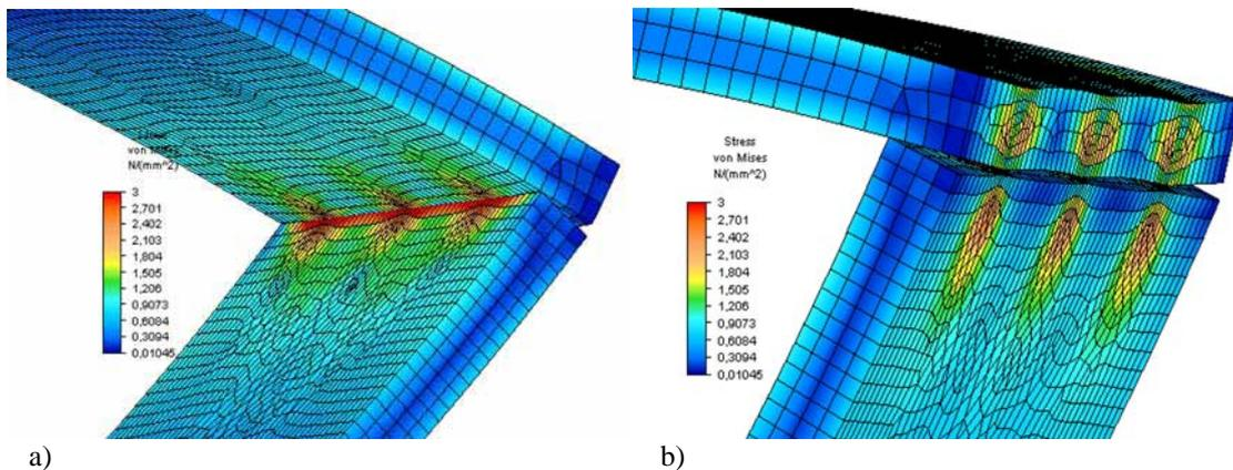
Fig. 5. Distribution of reduced stresses according to Mises in a dowel joint subjected to closing at the point of: a) board mutual pressure, b) pressure of fasteners on boards,  $\sigma_{\max} \approx 3 \text{ MPa}$
