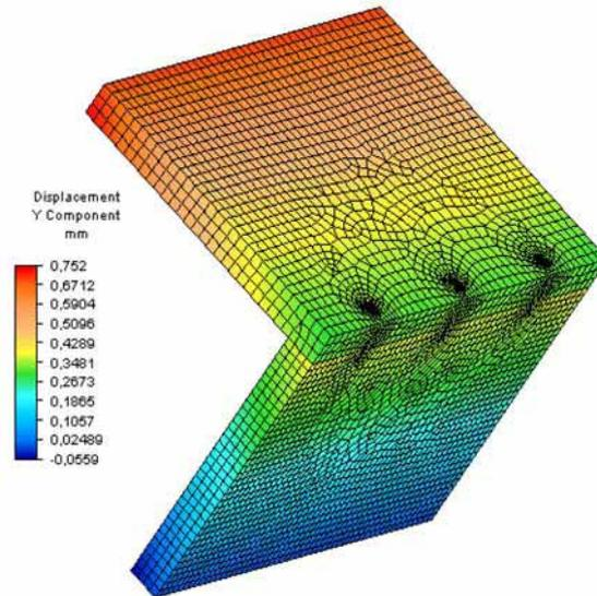
Fig. 8. Deflection value  $\delta_{1P}$  of the dowel joint subjected to closing,  $\delta_{1P(\max)}=0.75$  mm.
