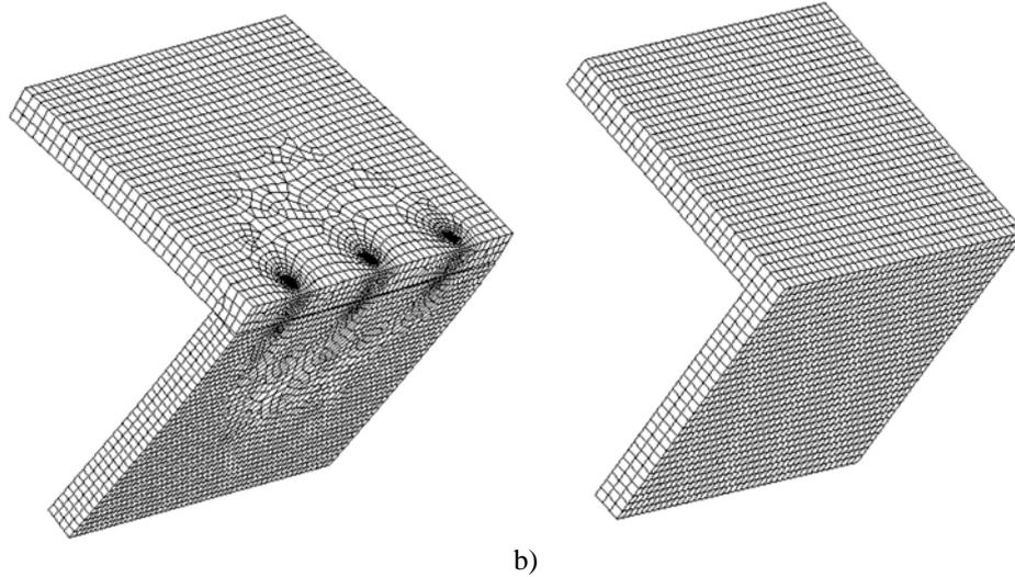
Fig. 3. Network of finite elements for a solid body model of angle joint containing: a) dowel pegs, b) element of a substitute modulus of rigidity  $E_z$
