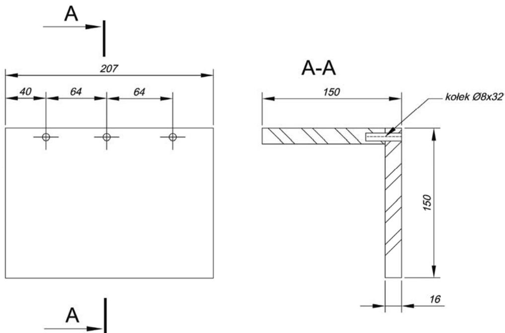
Fig. 1. Dowel joint
