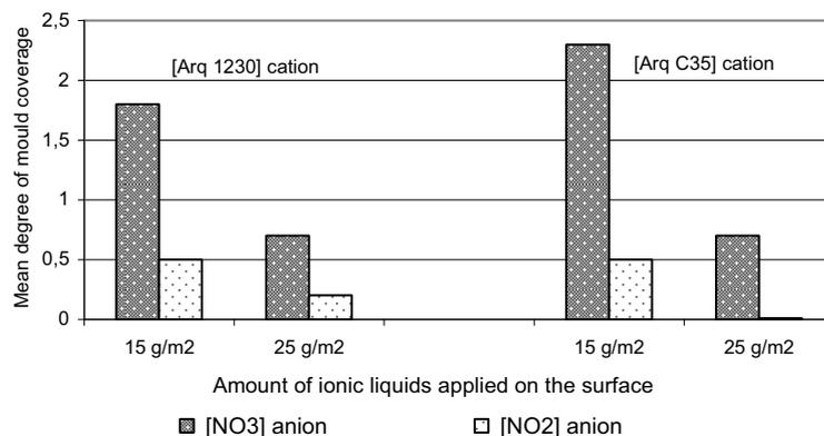
Fig.2. Comparison of average degree of mixture of mould coverage on the surface of wood protected with ammonium nitrates(III) and nitrates(V)
