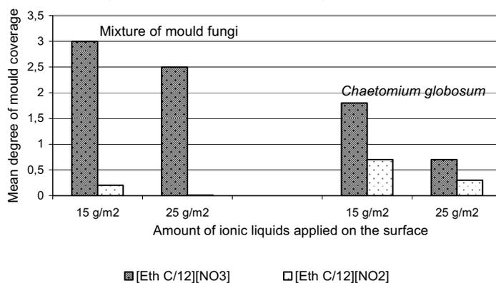
Fig.1. Comparison of average degree of mould coverage by tested fungi on the surface of wood protected with [Eth C/12] nitrate(III) and nitrate(V)
