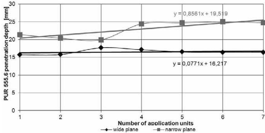
Fig. 4. Depth of the penetration area of the reinforcing agent in MDF.
