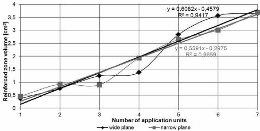
Fig. 5. Volume of the modified area in relation to the number of application units
