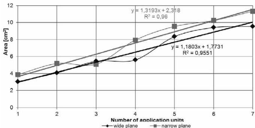
Fig. 6. Contact surface area of modified and non-modified layers of MDF.
