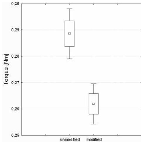
Fig.5. Level of torque for unmodified and modified wood during drilling parallel to annual rings.
