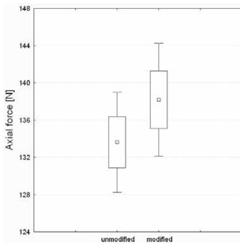
Fig.3. Level of axial force for unmodified and modified wood during drilling parallel to annual rings.
