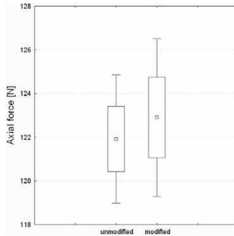
Fig.4. Level of axial force for modified and unmodified wood during drilling perpendicular to annual rings
