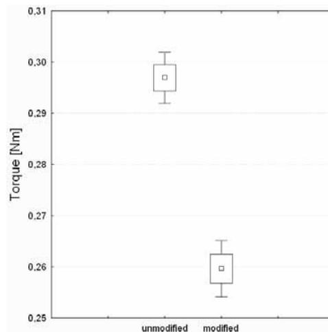
Fig.6. Level of torque for unmodified and modified wood during drilling perpendicular to annual rings.
