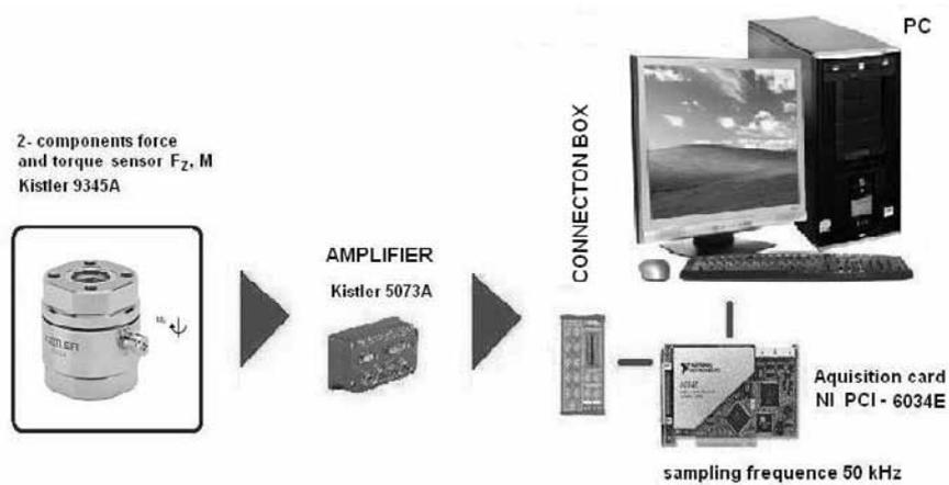
Fig.1. Measurement stand schema
