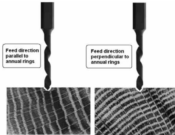
Fig.2. Variants of drilling in direction parallel and perpendicular to annual rings
