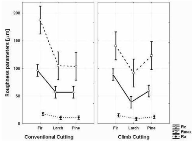
Fig.5. Influence of interactions between species of wood and kind of milling on machined surface roughness
