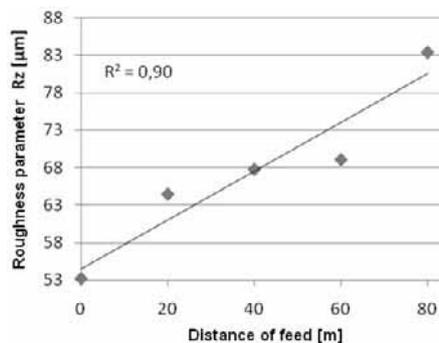
Fig.3. Dependency of machined surface roughness (parameter  $R_z$ ) from feed distance
