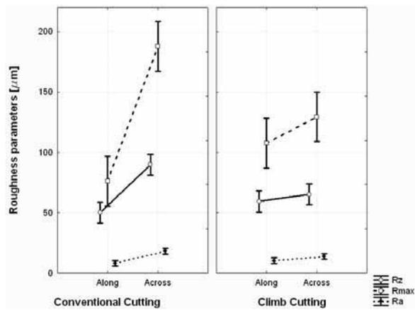
Fig.6. Influence of interactions between direction of milling and kind of milling on machined surface roughness
