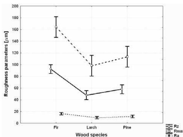
Fig.4. The influence of wood species on machined surface roughness
