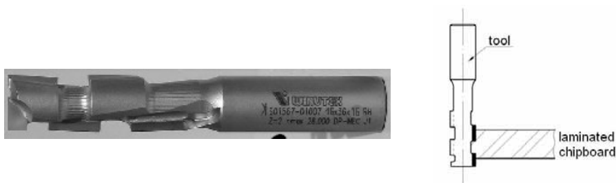
Fig.2. Router bit used in experiments and scheme of machining
