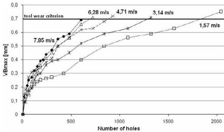
Fig.3. Curves of tool wear (dependency of indicator VBmax on number of drilled holes), it was graphically marked criterion of tool wear VBmax=0,7mm
