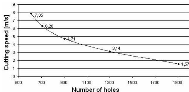
Fig.4. Number of holes made up to limit value of  $VB_{max} = 0,7\text{mm}$  for particular cutting speeds
