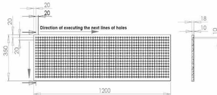
Fig.1. Schema of piece with cutting direction of successive hole rows
