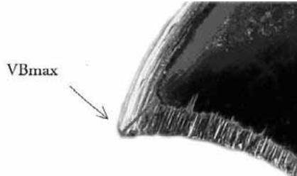
Fig. 2. Tool wear indicator VBmax
