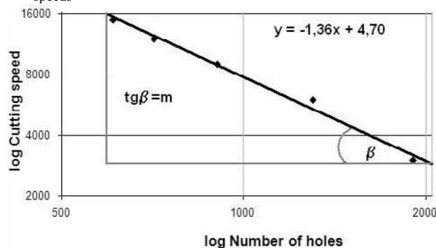
Fig.5. Dependence of tool life on cutting speed in logarithmic scale
