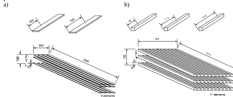
Fig. 1. Dimensions and location of probes for measuring temperature and moisture content during experiment: a) stack of boards b) stack of timber
