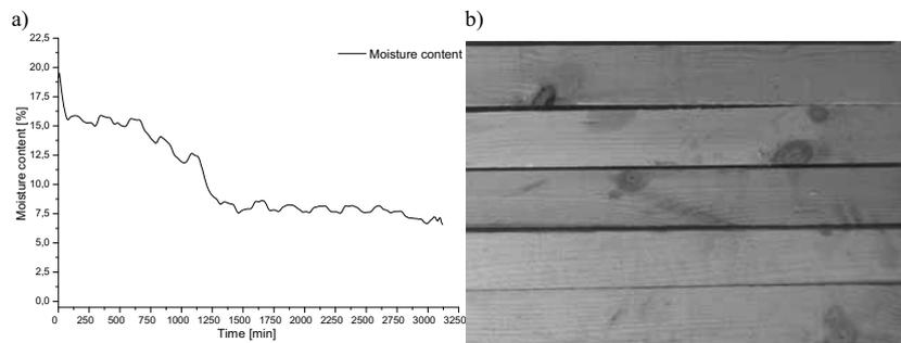
Fig. 2. The results of 7,0 cm x 7,0 cm pine lumber (Pinus L.) drying process using steam-gas mixture: a) time dependence of moisture content, b) fractures and colour changes of wood.
