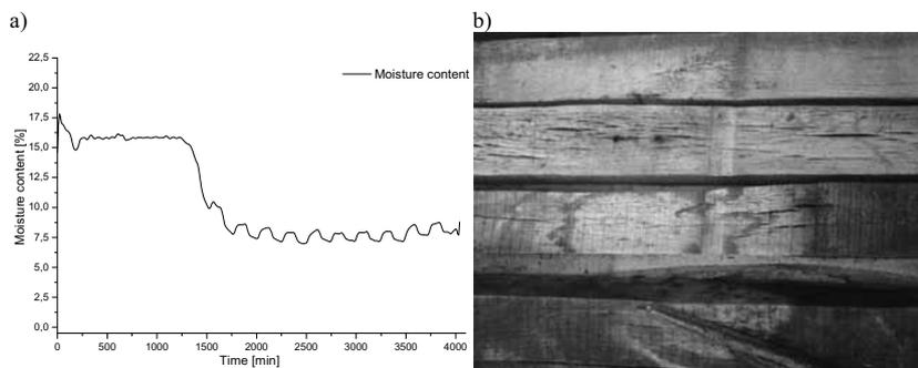
Fig. 3. The results of 7,0 cm x 7,0 cm pine lumber (*Quercus L.*) drying process using steam-gas mixture: a) time dependence of moisture content, b) fractures and colour changes of wood.\
