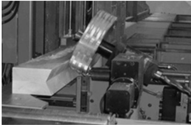
Fig. 7. Log milling - one can notice possibility of change of axial location of working spindle.
