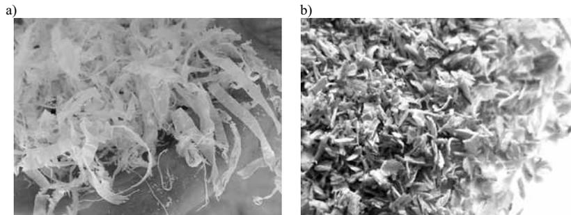
Fig. 1. Examples of chip forms formed during wood sawing: a) continuous chips, b) fine chips and sawdust
