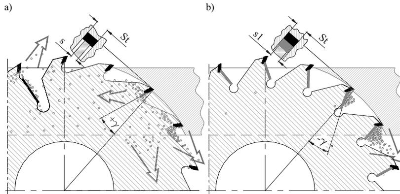
Fig. 2. Ways of chips transportation during sawing of wood with circular saw blades of the regular design (commonly used) (a) and circular saw blades with semi-closed gullets (b)
