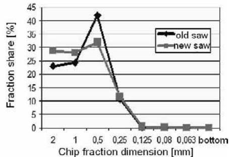
Fig. 3. Granulometric distribution of chips and sawdust obtained during sawing of pine with circular saw blades of the common design of gullets (old saw) and circular saw blades with semi-closed gullets (new saw)
