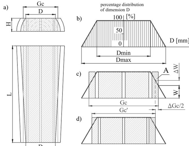
Fig. 2. Material with width and height changing along its length
